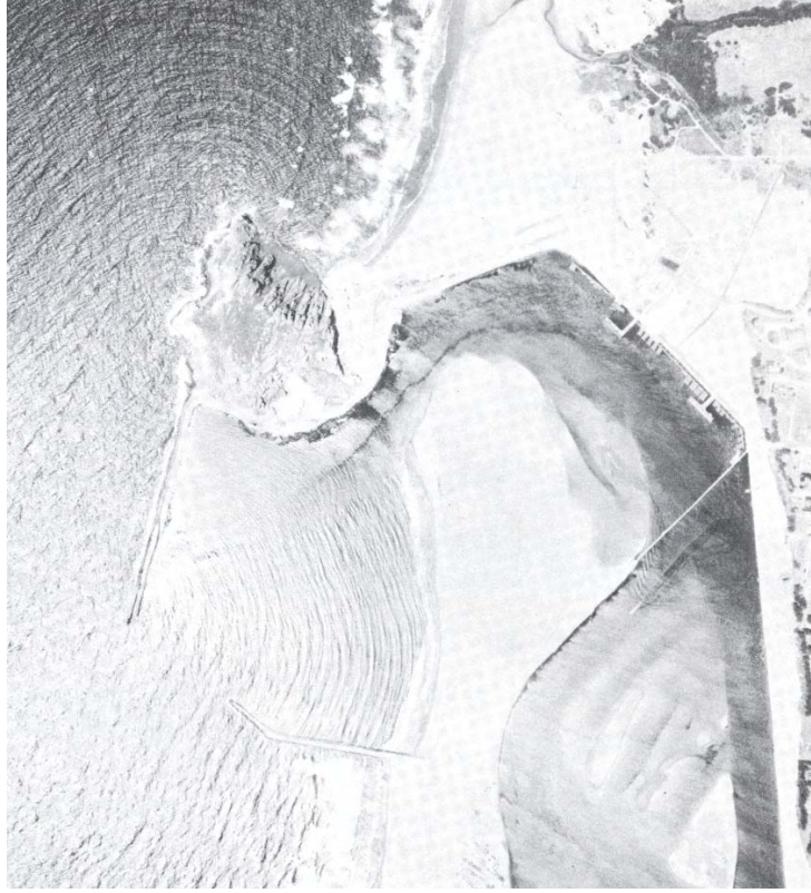
Figure 4.8: Diffraction around breakwater head.
