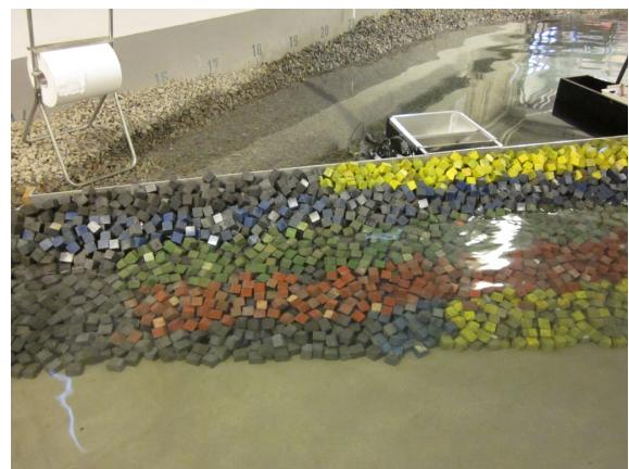
**Test no. 2.1.7 - SWL: +3.50, T<sub>p</sub>: 8 s, H<sub>m0</sub><sup>Gen</sup> = 4.87 m, H<sub>m0</sub><sup>Gen\*</sup> = 4.24 m**
