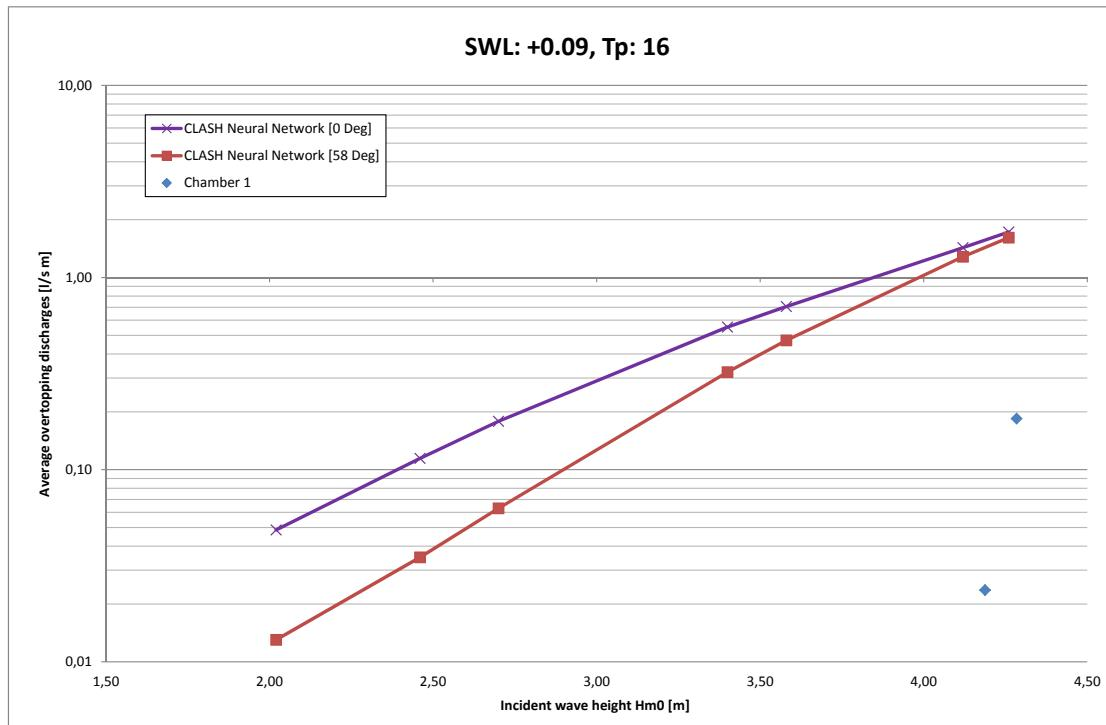
**Figure 9.2.** Average measured overtopping discharge for the caisson, and estimates from CLASH Neural Network.
