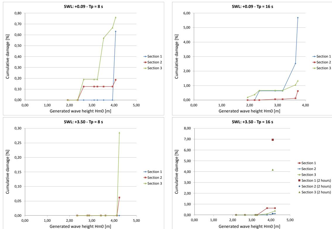
**Figure 8.2.** Cumulative damage of cube armour layer.
