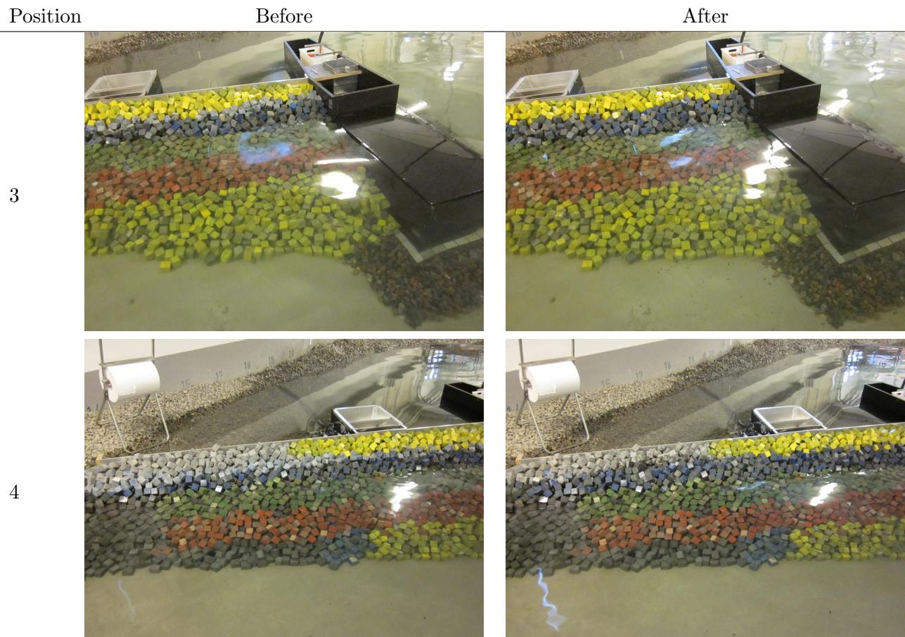
**Test no. 2.1.2 - SWL: +3.50, T<sub>p</sub>: 8 s, H<sub>m0</sub><sup>Gen</sup> = 3.14 m, H<sub>m0</sub><sup>Gen\*</sup> = 2.73 m**
