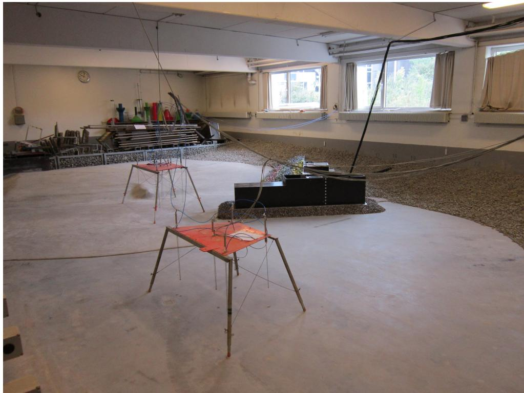
**Figure 2.18.** The wave gauge arrays as positioned in the basin.
