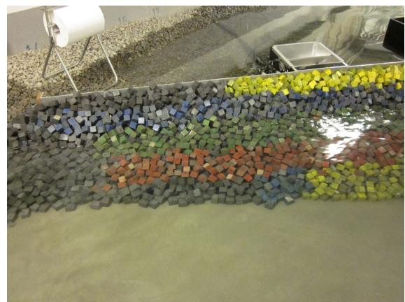
**Test no. 2.2.6 - SWL: +3.50, T<sub>p</sub>: 16 s, H<sub>m0</sub><sup>Gen</sup> = 4.84 m, H<sub>m0</sub><sup>Gen\*</sup> = 4.21 m**
