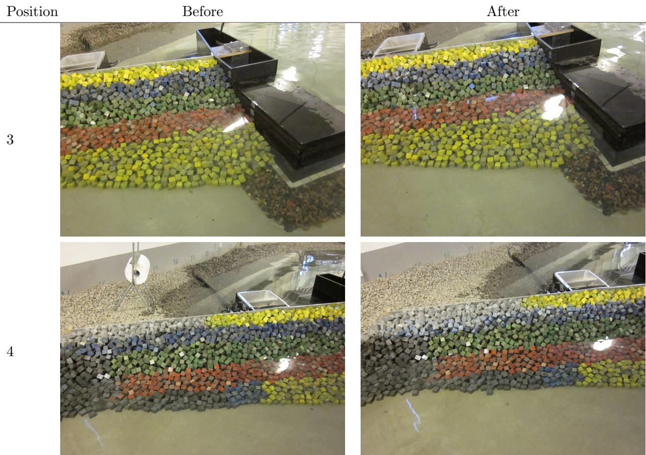
**Test no. 1.2.2 - SWL: +0.09, T<sub>p</sub>: 16 s, H<sub>m0</sub><sup>Gen</sup> = 2.51 m, H<sub>m0</sub><sup>Gen\*</sup> = 2.18 m**
