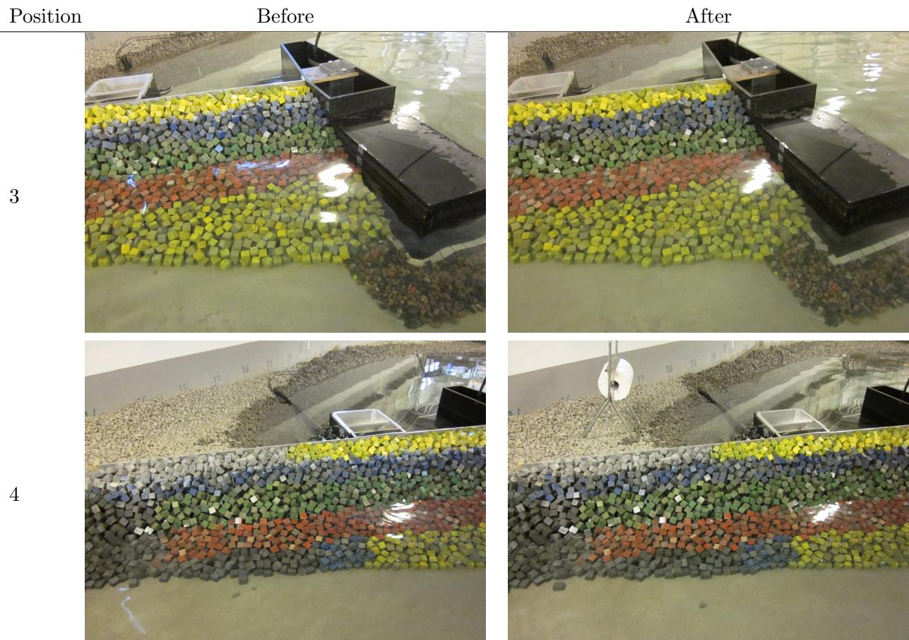
**Test no. 1.2.4 - SWL: +0.09, T<sub>p</sub>: 16 s, H<sub>m0</sub><sup>Gen</sup> = 3.35 m, H<sub>m0</sub><sup>Gen\*</sup> = 2.91 m**
