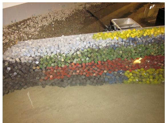
**Test no. 1.1.3 - SWL: +0.09, T<sub>p</sub>: 8 s, H<sub>m0</sub><sup>Gen</sup> = 3.03 m, H<sub>m0</sub><sup>Gen\*</sup> = 2.63 m**
