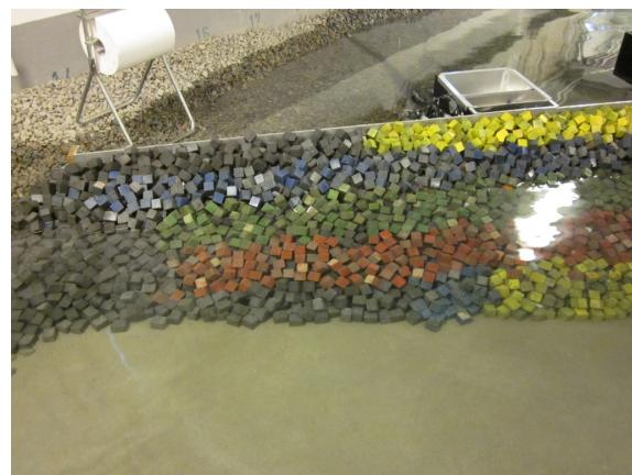
**Test no. 2.2.5 - SWL: +3.50, T<sub>p</sub>: 16 s, H<sub>m0</sub><sup>Gen</sup> = 4.36 m, H<sub>m0</sub><sup>Gen\*</sup> = 3.80 m**
