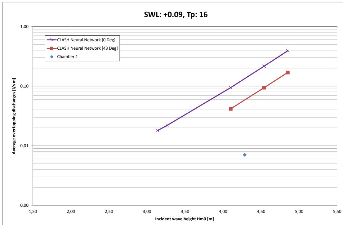
**Figure 9.5.** Average measured overtopping discharge on the rubble mound, and estimates from CLASH Neural Network.
