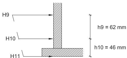
The uplift force is estimated by assuming a triangular distribution of the pressure underneath the caisson. The pressure  $V_1$  is assumed equal to  $H_{11}$  and the pressure at the heel of the caisson is assumed to be zero.
