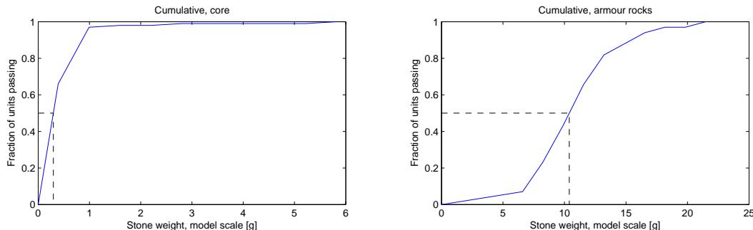
**Figure 2.13.** Grain curves of materials.
