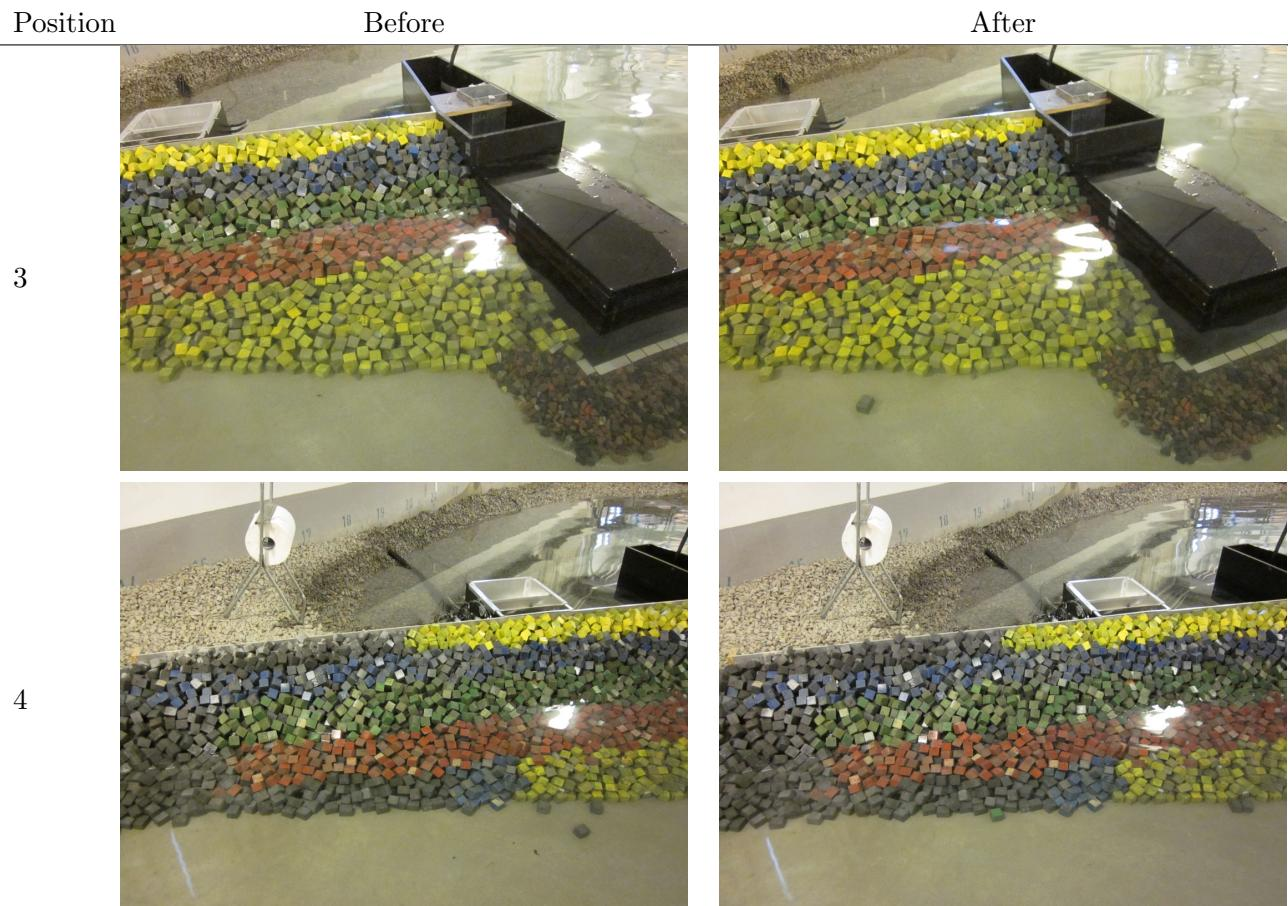
**Test no. 1.2.7 - SWL: +0.09, T<sub>p</sub>: 16 s, H<sub>m0</sub><sup>Gen</sup> = 4.28 m, H<sub>m0</sub><sup>Gen\*</sup> = 3.73 m**
