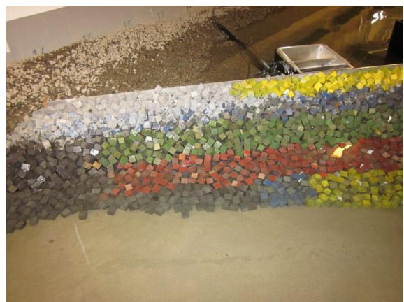
**Test no. 1.1.4 - SWL: +0.09, T<sub>p</sub>: 8 s, H<sub>m0</sub><sup>Gen</sup> = 3.57 m, H<sub>m0</sub><sup>Gen\*</sup> = 3.10 m**
