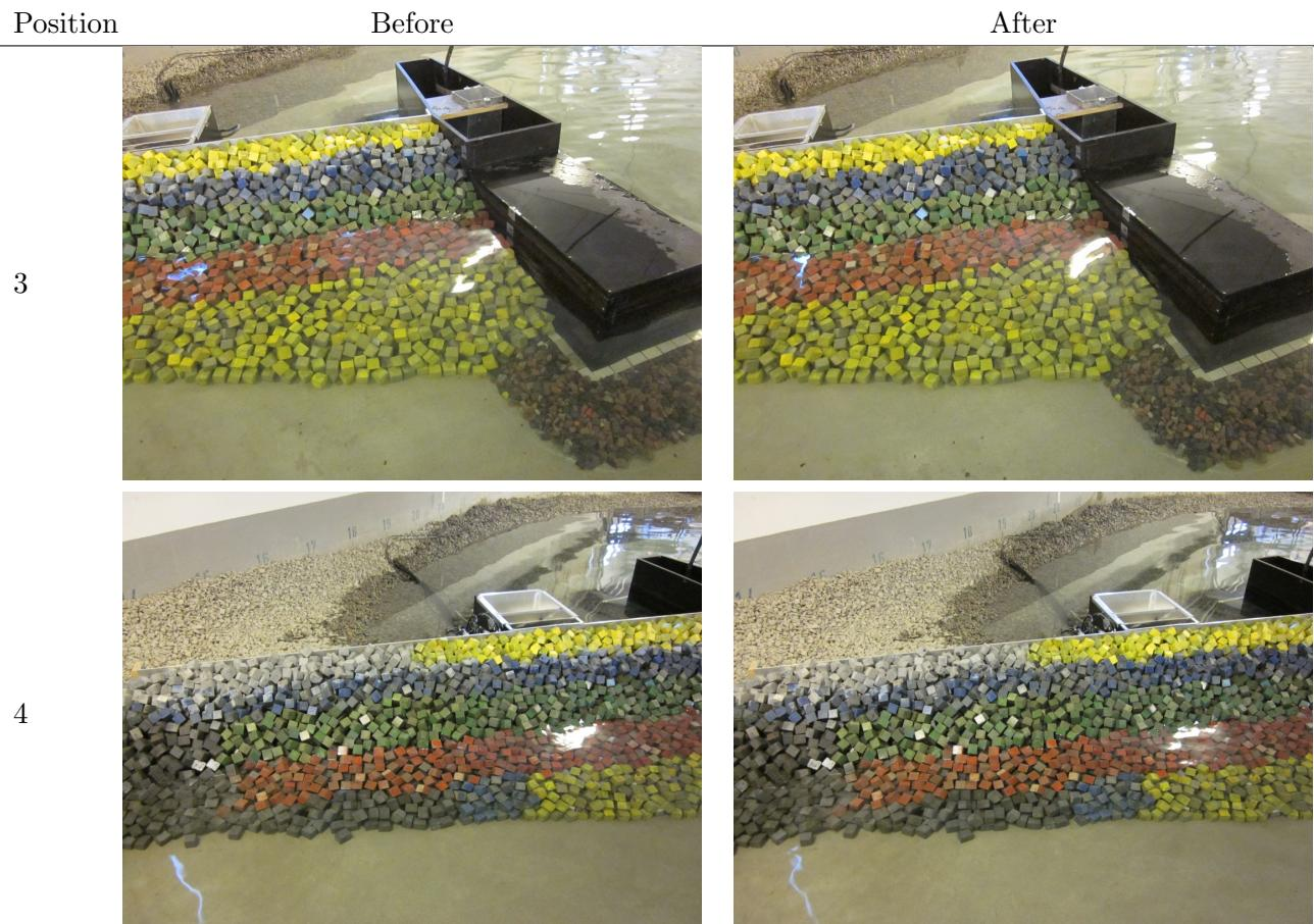
**Test no. 1.1.6 - SWL: +0.09,  $T_p$ : 8 s,  $H_{m0}^{Gen} = 4.06$  m,  $H_{m0}^{Gen*} = 3.53$  m**
