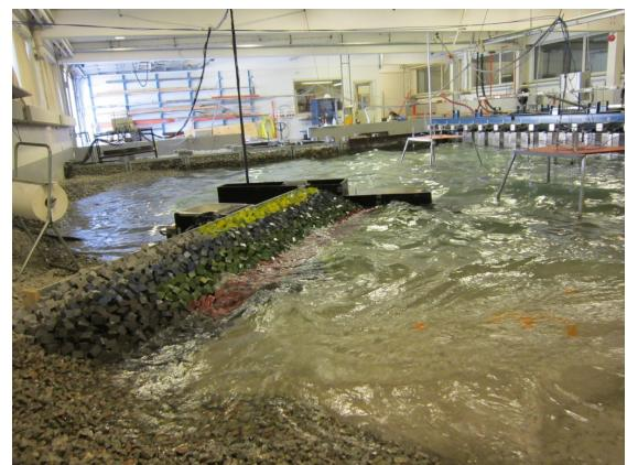
**Figure 2.8.** Picture of the model with water and waves.
