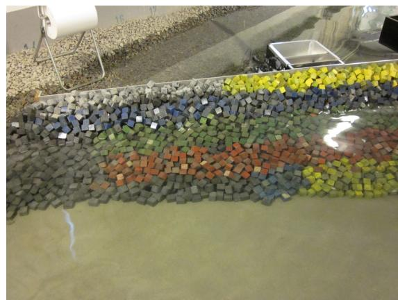
**Test no. 2.2.2 - SWL: +3.50, T<sub>p</sub>: 16 s, H<sub>m0</sub><sup>Gen</sup> = 3.04 m, H<sub>m0</sub><sup>Gen\*</sup> = 2.64 m**
