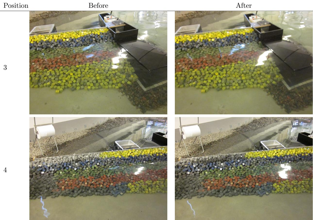
**Test no. 2.1.3 - SWL: +3.50, T<sub>p</sub>: 8 s, H<sub>m0</sub><sup>Gen</sup> = 3.31 m, H<sub>m0</sub><sup>Gen\*</sup> = 2.88 m**
