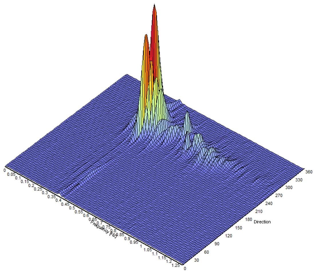
**Figure 3.1.** 3D variance spectrum of measured waves.
