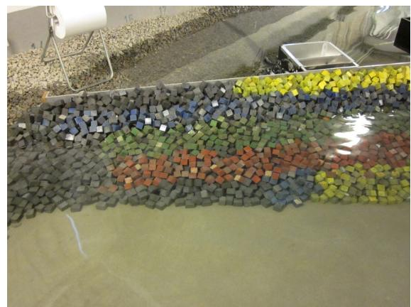
**Test no. 2.2.4 - SWL: +3.50, T<sub>p</sub>: 16 s, H<sub>m0</sub><sup>Gen</sup> = 3.77 m, H<sub>m0</sub><sup>Gen\*</sup> = 3.27 m**
