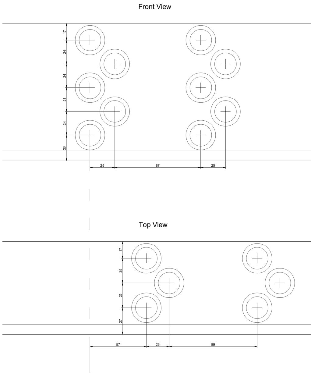
**Figure 2.15.** Pressure gauge locations at the crown wall on the rubble mound breakwater (annotations in millimetres in model scale).
