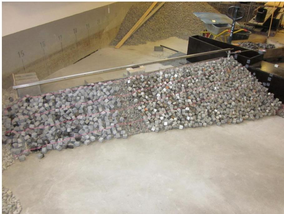
**Figure 2.14.** Inner armour layer. Note the cubes were substituted with parallelepipeds armour block in the inner layer on a stretch of the rubble mound.
