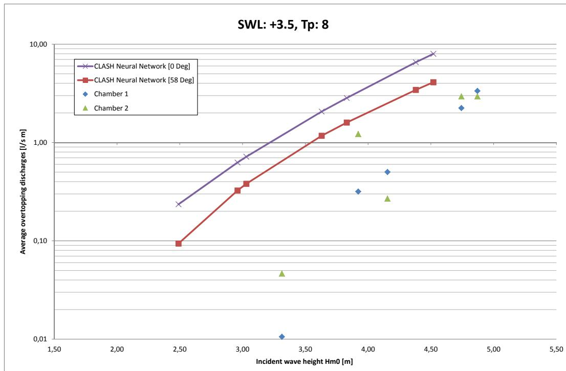
**Figure 9.3.** Average measured overtopping discharge for the caisson, and estimates from CLASH Neural Network.
