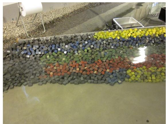
**Test no. 2.2.3 - SWL: +3.50, T<sub>p</sub>: 16 s, H<sub>m0</sub><sup>Gen</sup> = 3.66 m, H<sub>m0</sub><sup>Gen\*</sup> = 3.18 m**
