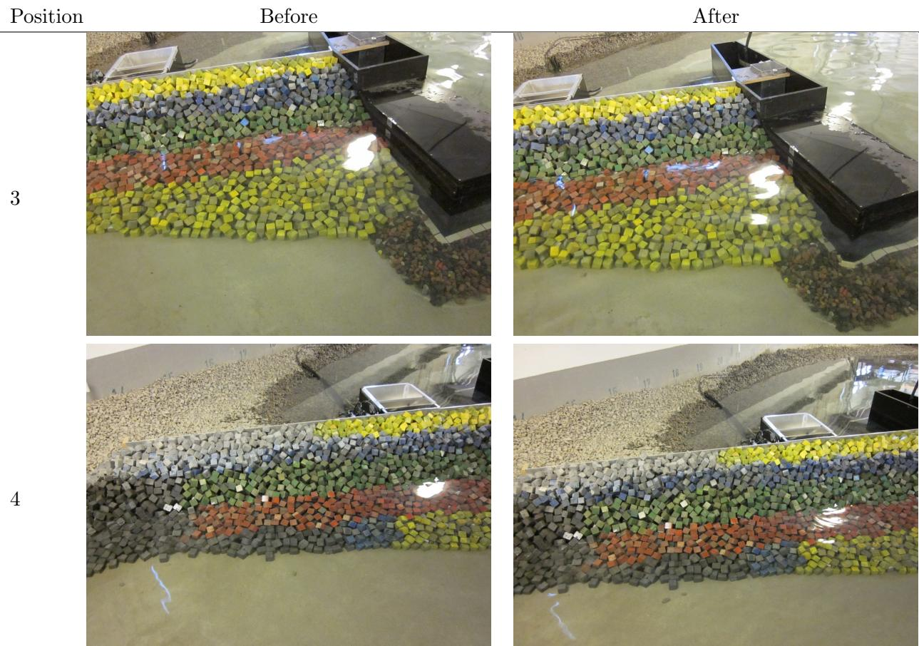
**Test no. 1.2.3 - SWL: +0.09, T<sub>p</sub>: 16 s, H<sub>m0</sub><sup>Gen</sup> = 2.70 m, H<sub>m0</sub><sup>Gen\*</sup> = 2.35 m**
