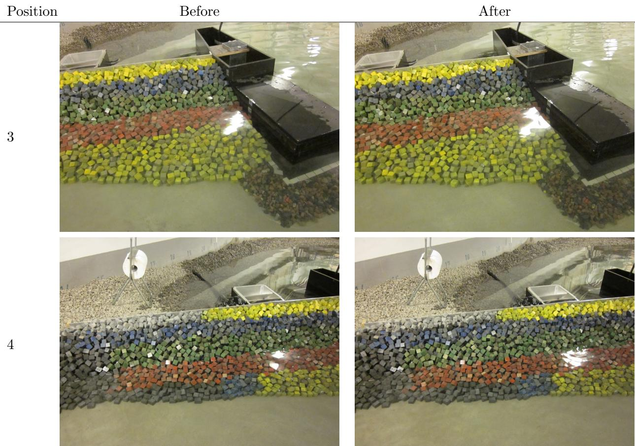
**Test no. 1.2.5 - SWL: +0.09, T<sub>p</sub>: 16 s, H<sub>m0</sub><sup>Gen</sup> = 3.66 m, H<sub>m0</sub><sup>Gen\*</sup> = 3.18 m**
