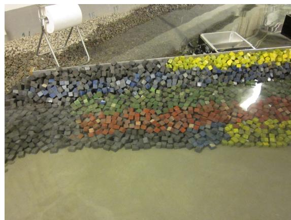
**Test no. (2.2.6) - SWL: +3.50, T<sub>p</sub>: 16 s, H<sub>m0</sub><sup>Gen</sup> = 4.70 m,
