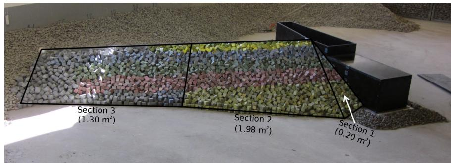
**Figure 8.1.** Sections used for rubble-mound armour cube stability.
