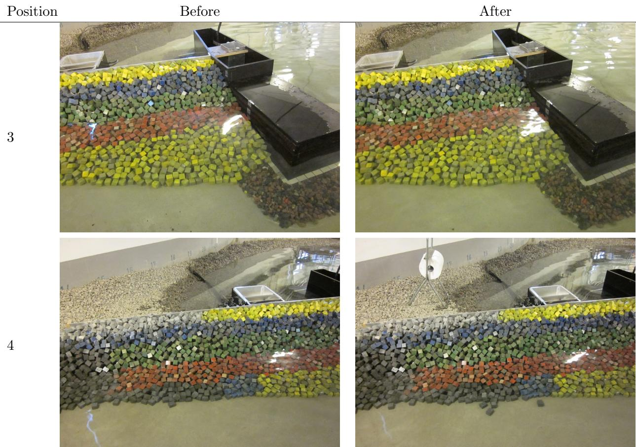
**Test no. 1.1.7 - SWL: +0.09, T<sub>p</sub>: 8 s, H<sub>m0</sub><sup>Gen</sup> = 4.52 m, H<sub>m0</sub><sup>Gen\*</sup> = 3.93 m**
