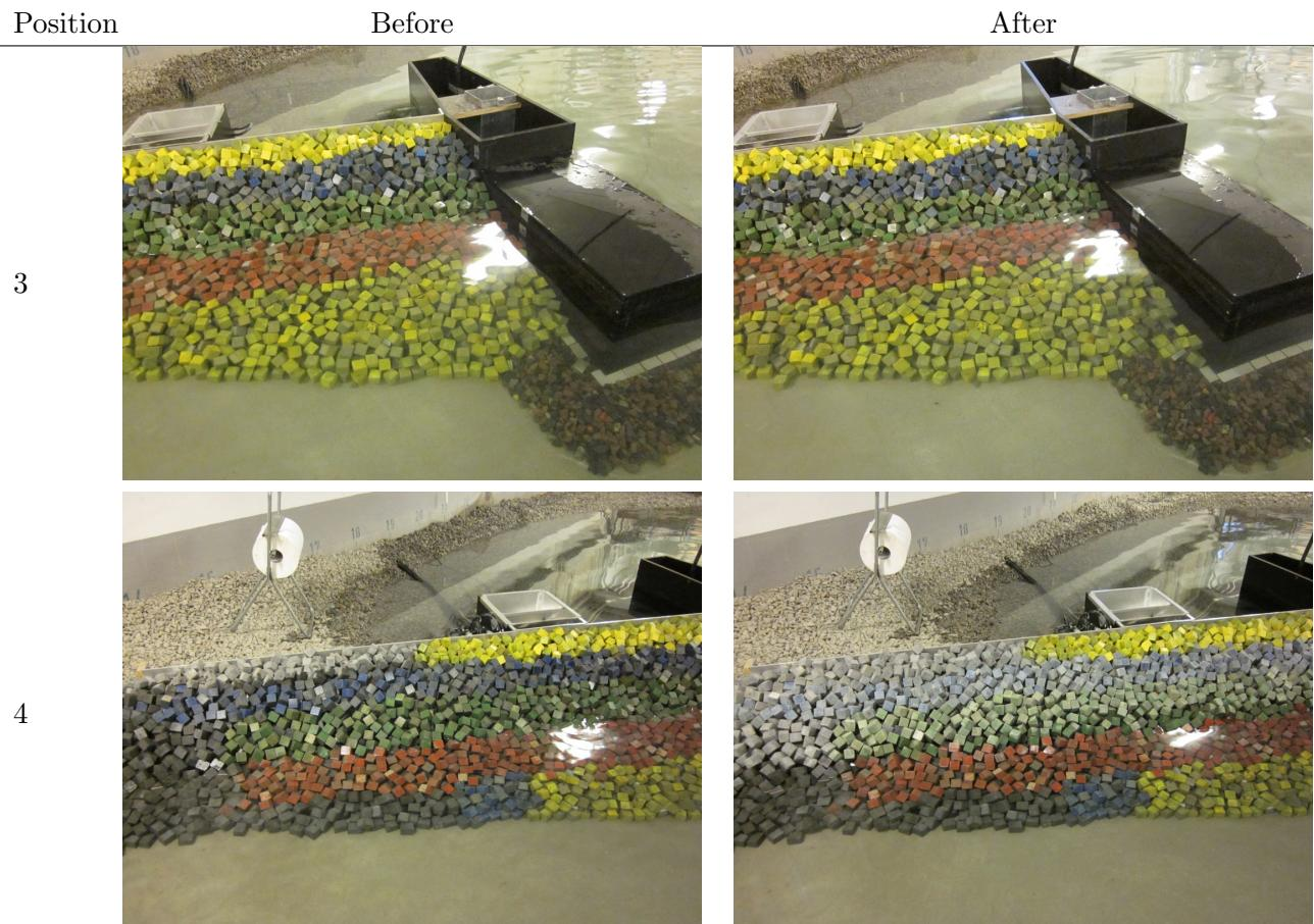
**Test no. 1.2.6 - SWL: +0.09, T<sub>p</sub>: 16 s, H<sub>m0</sub><sup>Gen</sup> = 4.19 m, H<sub>m0</sub><sup>Gen\*</sup> = 3.64 m**
