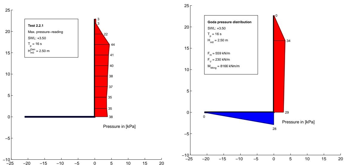
**Test no. 2.2.2, SWL: +3.50,  $T_p$ : 16 s,  $H_{m0}^{Gen} = 3.04$  m**
