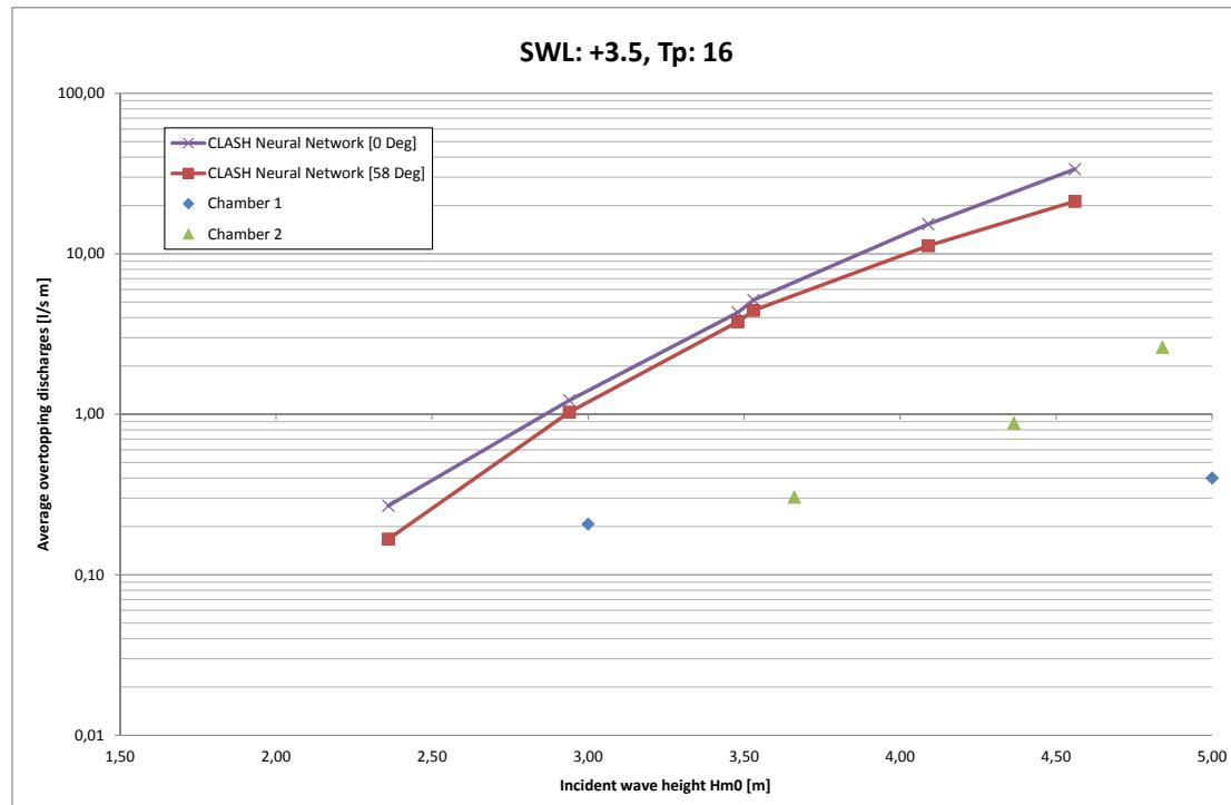
**Figure 9.4.** Average measured overtopping discharge for the caisson, and estimates from CLASH Neural Network.
