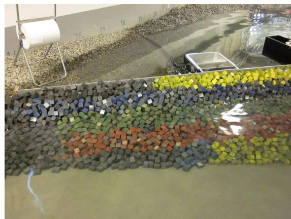
**Test no. 2.1.6 - SWL: +3.50, T<sub>p</sub>: 8 s, H<sub>m0</sub><sup>Gen</sup> = 4.74 m, H<sub>m0</sub><sup>Gen\*</sup> = 4.12 m**
