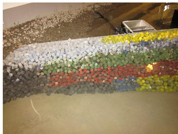
**Test no. 1.1.2 - SWL: +0.09, T<sub>p</sub>: 8 s, H<sub>m0</sub><sup>Gen</sup> = 2.72 m, H<sub>m0</sub><sup>Gen\*</sup> = 2.36 m**
