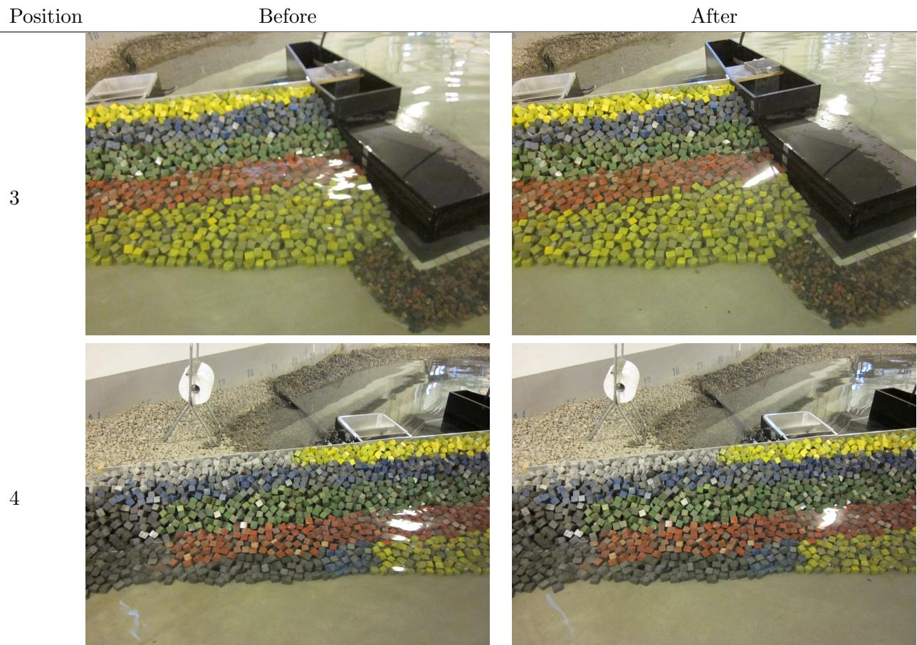
**Test no. 1.1.7 - SWL: +0.09,  $T_p$ : 8 s,  $H_{m0}^{Gen} = 4.68$  m,  $H_{m0}^{Gen*} = 4.07$  m**
