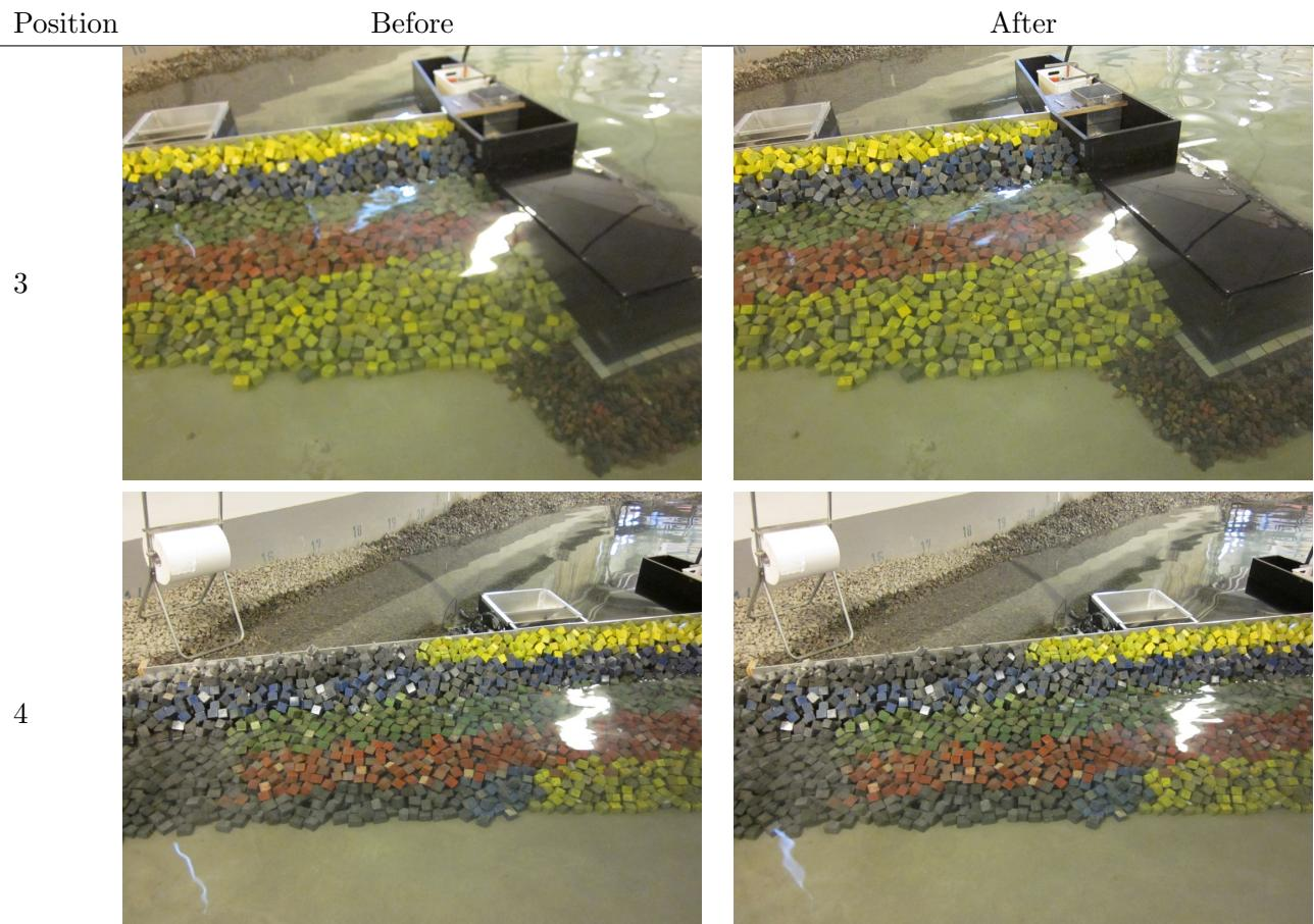
**Test no. 2.1.4 - SWL: +3.50, T<sub>p</sub>: 8 s, H<sub>m0</sub><sup>Gen</sup> = 3.92 m, H<sub>m0</sub><sup>Gen\*</sup> = 3.41 m**
