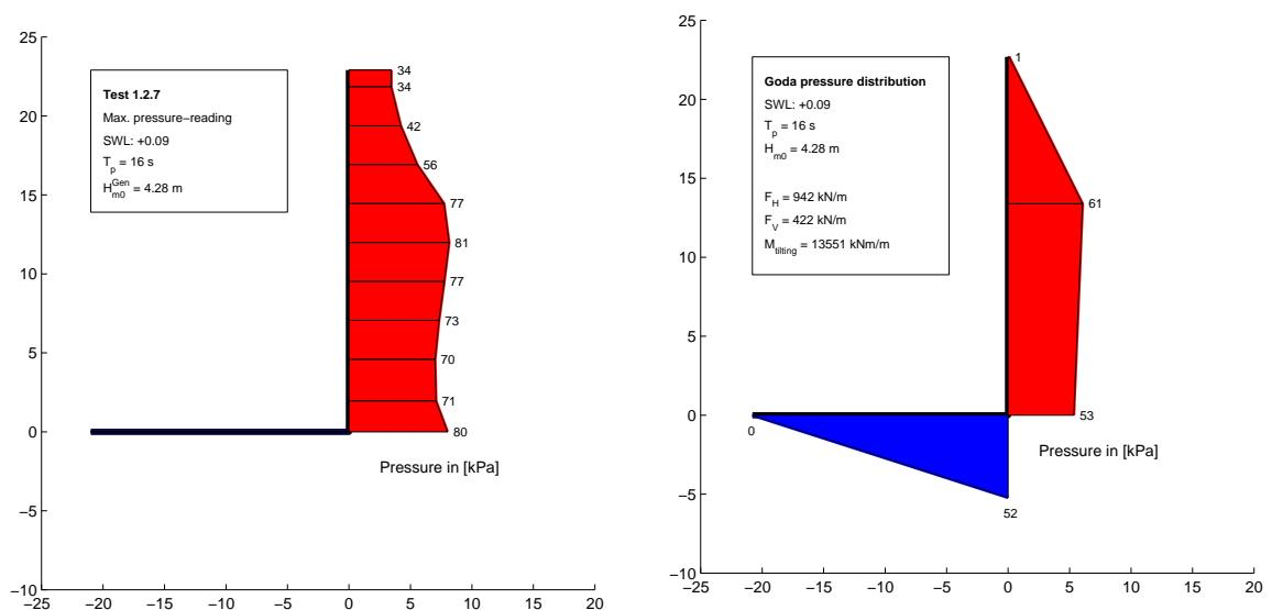
**Test no. 2.1.1, SWL: +3.50,  $T_p$ : 8 s,  $H_{m0}^{Gen} = 2.70$  m**
