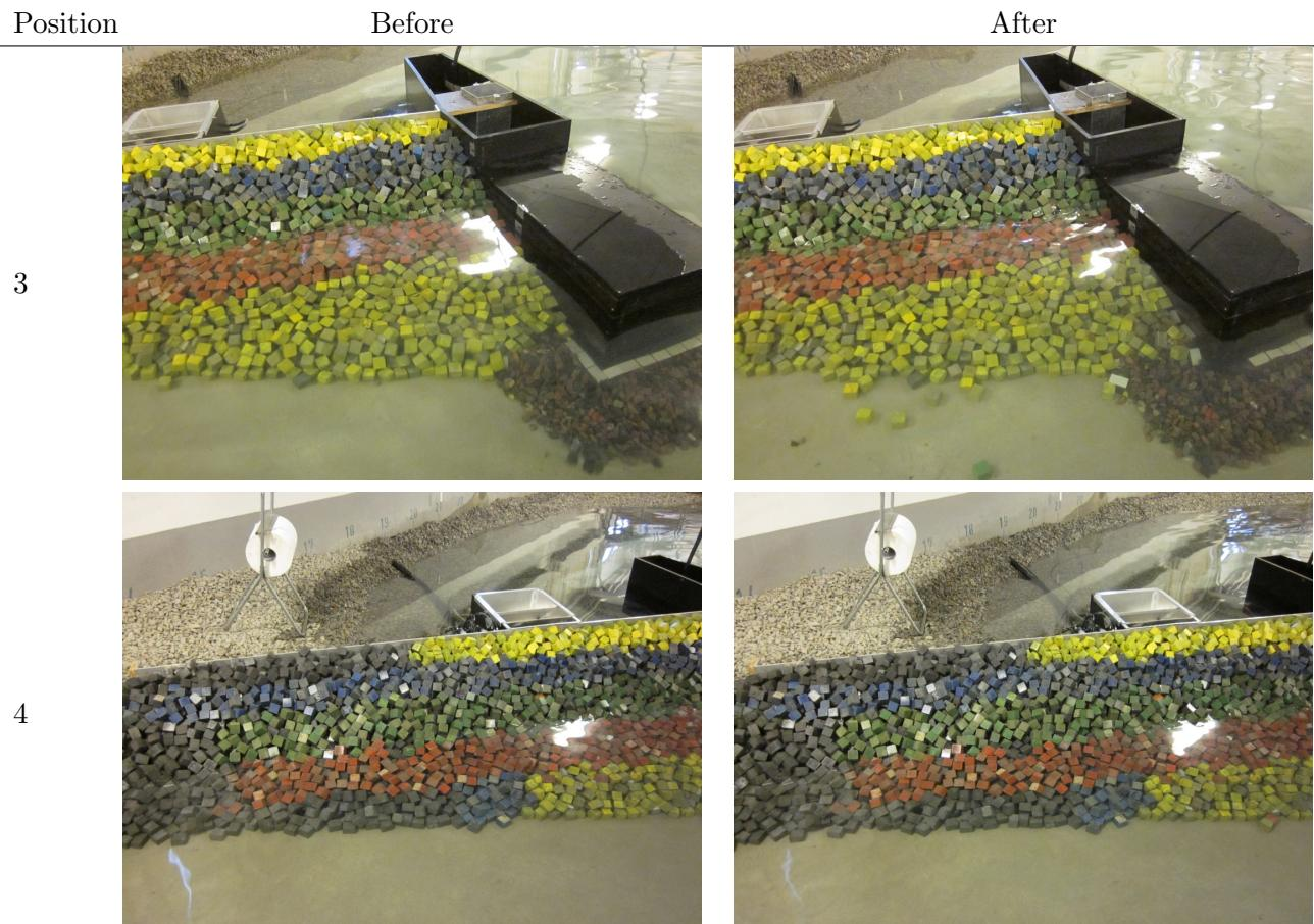
**Test no. 2.1.1 - SWL: +3.50, T<sub>p</sub>: 8 s, H<sub>m0</sub><sup>Gen</sup> = 2.70 m, H<sub>m0</sub><sup>Gen\*</sup> = 2.34 m**
