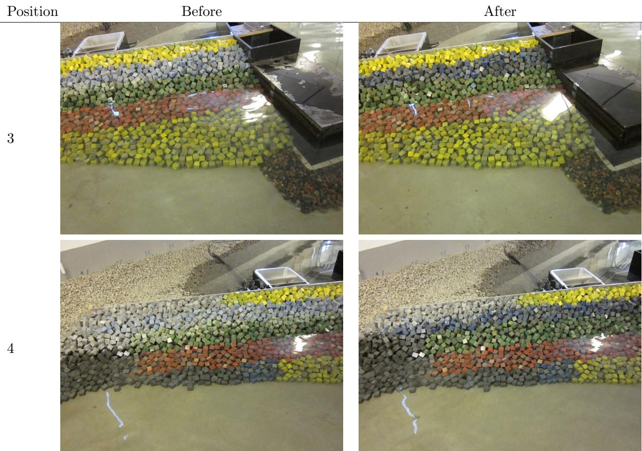
**Test no. 1.1.5 - SWL: +0.09,  $T_p$ : 8 s,  $H_{m0}^{Gen} = 3.74$  m,  $H_{m0}^{Gen*} = 3.25$  m**
