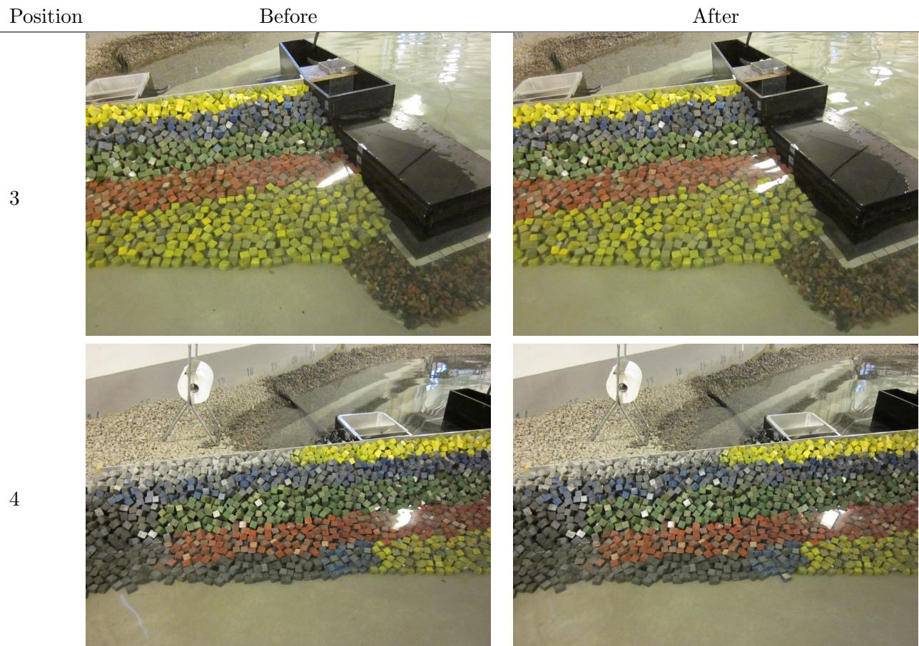
**Test no. 1.2.1 - SWL: +0.09, T<sub>p</sub>: 16 s, H<sub>m0</sub><sup>Gen</sup> = 2.22 m, H<sub>m0</sub><sup>Gen\*</sup> = 1.93 m**
