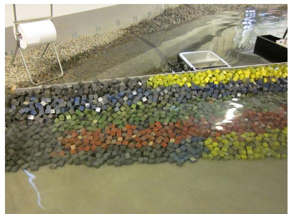
**Test no. 2.1.5 - SWL: +3.50, T<sub>p</sub>: 8 s, H<sub>m0</sub><sup>Gen</sup> = 4.15 m, H<sub>m0</sub><sup>Gen\*</sup> = 3.61 m**
