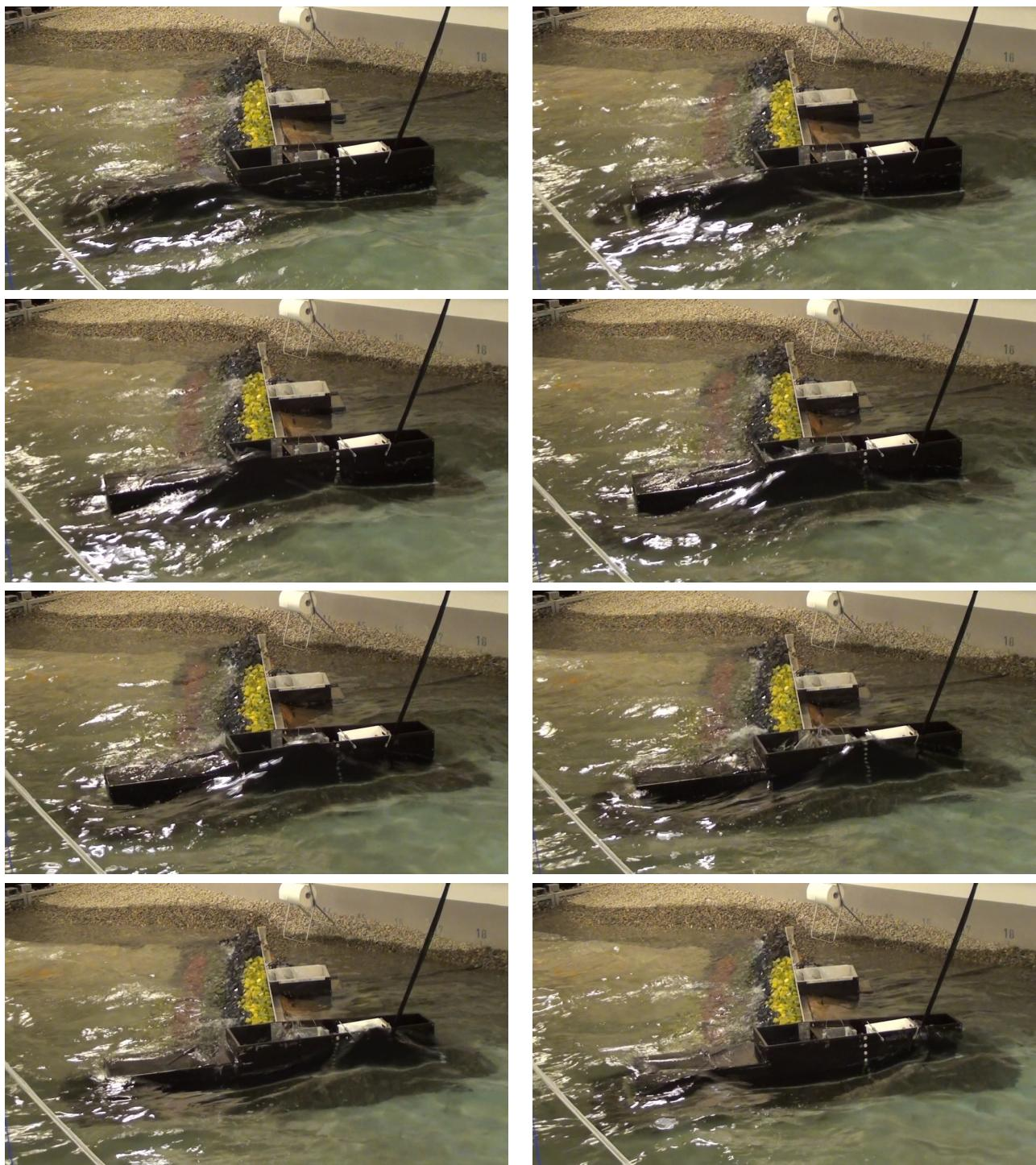
**Test no. 2.2.6, SWL: +3.50,  $T_p$ : 16 s,  $H_{m0}^{Gen}$ : 4.84 m**
