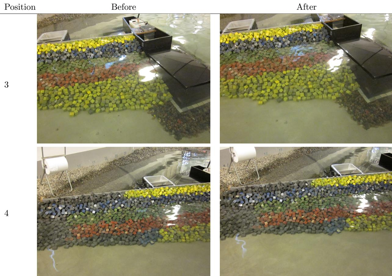
**Test no. 2.2.1 - SWL: +3.50, T<sub>p</sub>: 16 s, H<sub>m0</sub><sup>Gen</sup> = 2.50 m, H<sub>m0</sub><sup>Gen\*</sup> = 2.17 m**
