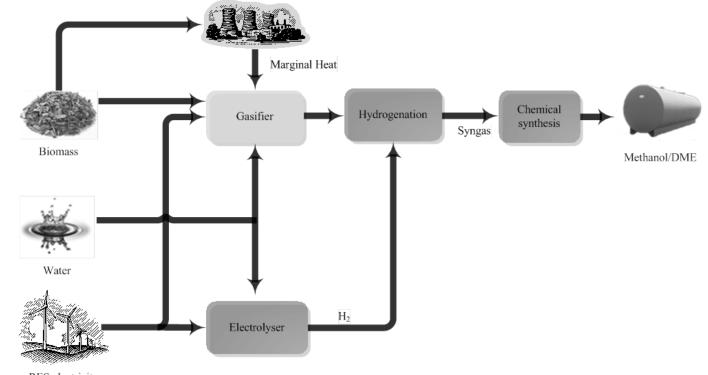
CO<sub>2</sub> recycling pathways (CO<sub>2</sub> hydrogenation and co-electrolysis) do not require any direct biomass input, instead they use emissions from the biomass used in the heat and power sector combined with electrolysis.
