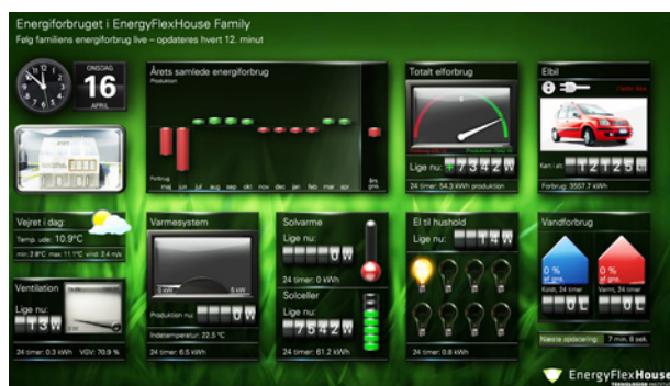
Fig. 22. In the demonstration project EnergyFlexHouse at the Danish Technological Institute, indoor environment parameters and energy use are visualised for the user. The system is user controlled via computer apps.
