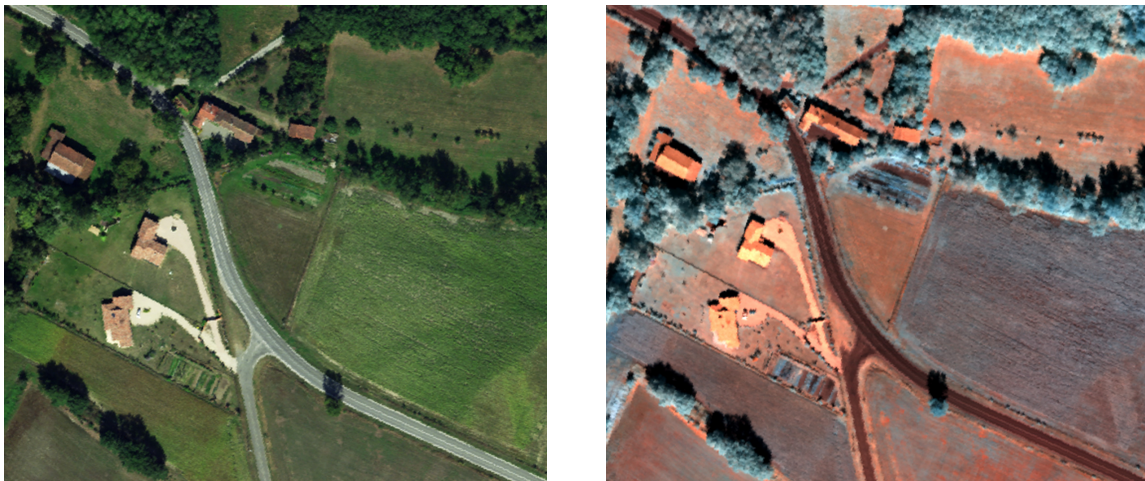
Figure 1 RGB representation of georeferenced and radiometrically calibrated image. VNIR (left), SWIR (right).
