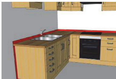
Good practice (uninterrupted resilient layer)
