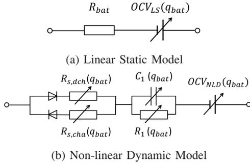
Fig. 4: Battery cell's Equivalent Circuit Models
