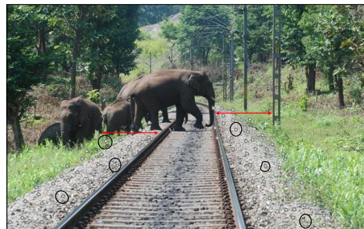
Fig. 1. Passive sensing nodes (some encircled), red arrows - the maximum possible width of electromagnetic board
