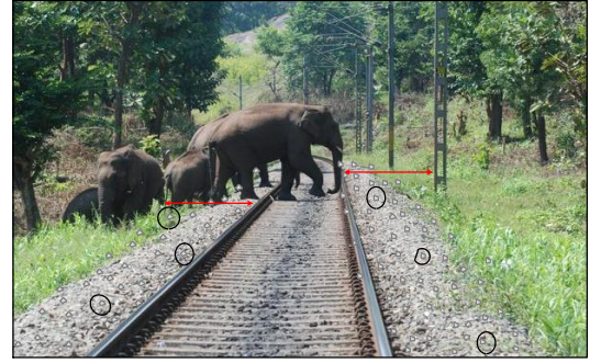
Fig. 1. Passive sensing nodes (some encircled), red arrows - the maximum possible width of electromagnetic board
