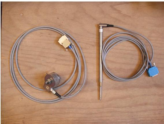
Figure 27: Force and displacement transducer
