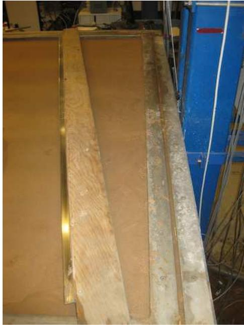
Figure 10: Lath used to smooth the soil surface
