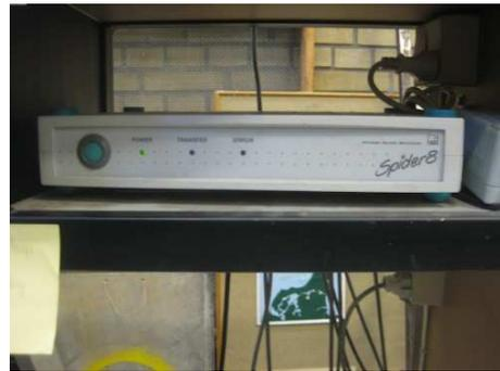
Figure 5: Data acquisition system (Spider 8)
