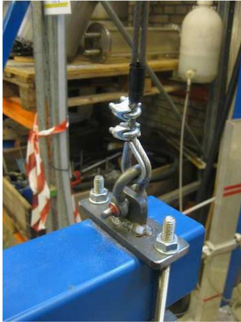
Figure 22: Connection between the hinged beam and the safety cable
