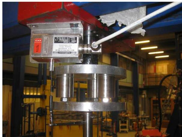
Figure 14: CPT displacement transducer
