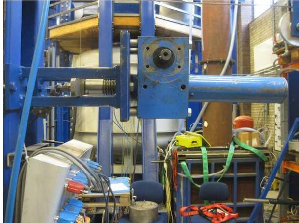
Figure 23: Static loading screw jack
