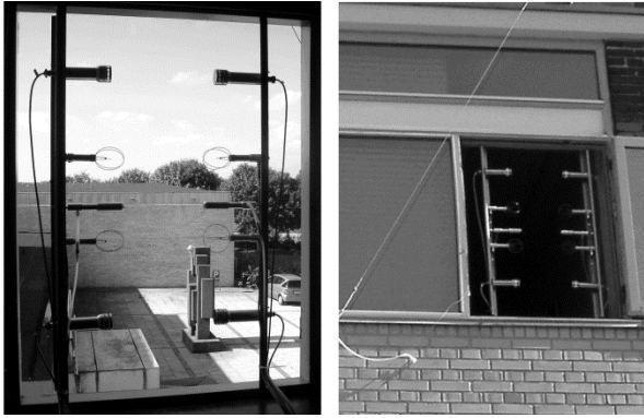
Figure 12. Measurement of velocity profiles in an opening. View from inside (left), view from outside (right).
