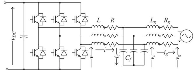
Fig. 1. An  $LCL$ -filter based three-phase active rectifier.
