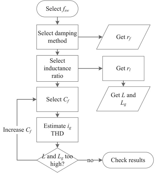
Fig. 5. Design flow for the  $LCL$ -filter.
