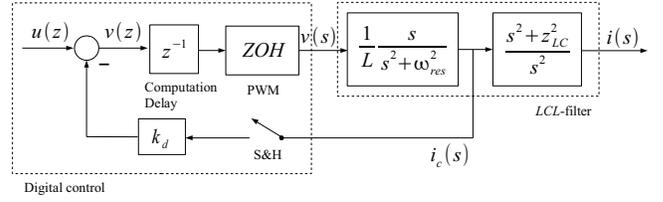
Fig. 4. Digital implementation of the capacitor current feedback.
