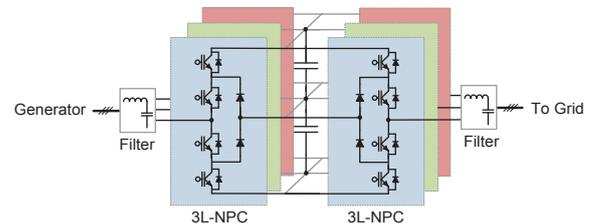
Fig. 11. 3L-NPC Back-to-Back (3L-NPC BTB) converter for WTS.
