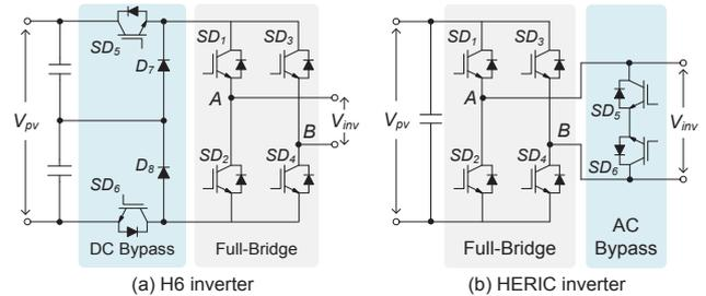
Fig. 14. Two transformerless PV inverters (H6 and HERIC) [25], [27].
