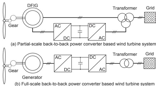
Fig. 9. Two dominant power electronics based WTS configurations.
