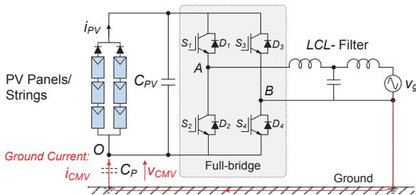
Fig. 13. Single-phase full-bridge PV inverter with an LCL-filter.
