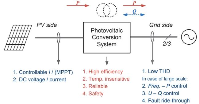
Fig. 8. Demands for PV power conversion system.
