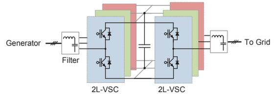
Fig. 10. 2L-VSC Back-to-Back (2L-VSC BTB) converter for WTS.
