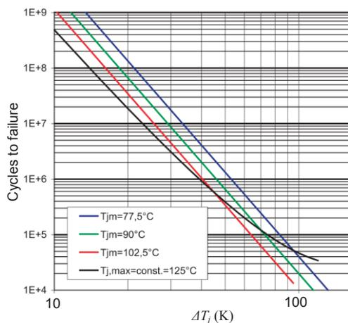
Fig. 24. Illustration of industrial standard cycles to failure vs.  $\Delta T_j$  of IGBT module by Semikron [65].
