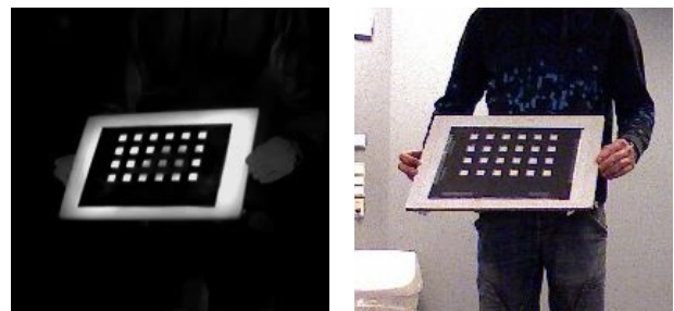
Fig. 12 Thermal and visible image of a calibration chessboard consisting of two cardboard sheets, where only the white layer has been heated before assembling.
