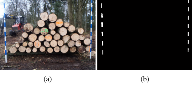
Figure 3: Result of marker segmentation. The input image (a) and the resulting binary map after thresholding and applying morphological operations (b)
