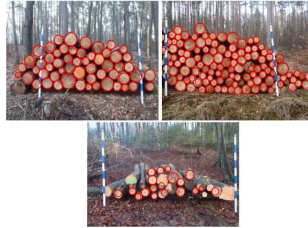
Figure 8: Visualized performance of the proposed system: top-left: good performance, top-right: medium performance, and bottom: bad performance. Detected wood logs are illustrated by the superimposed red circles indicating detected position and radius.
