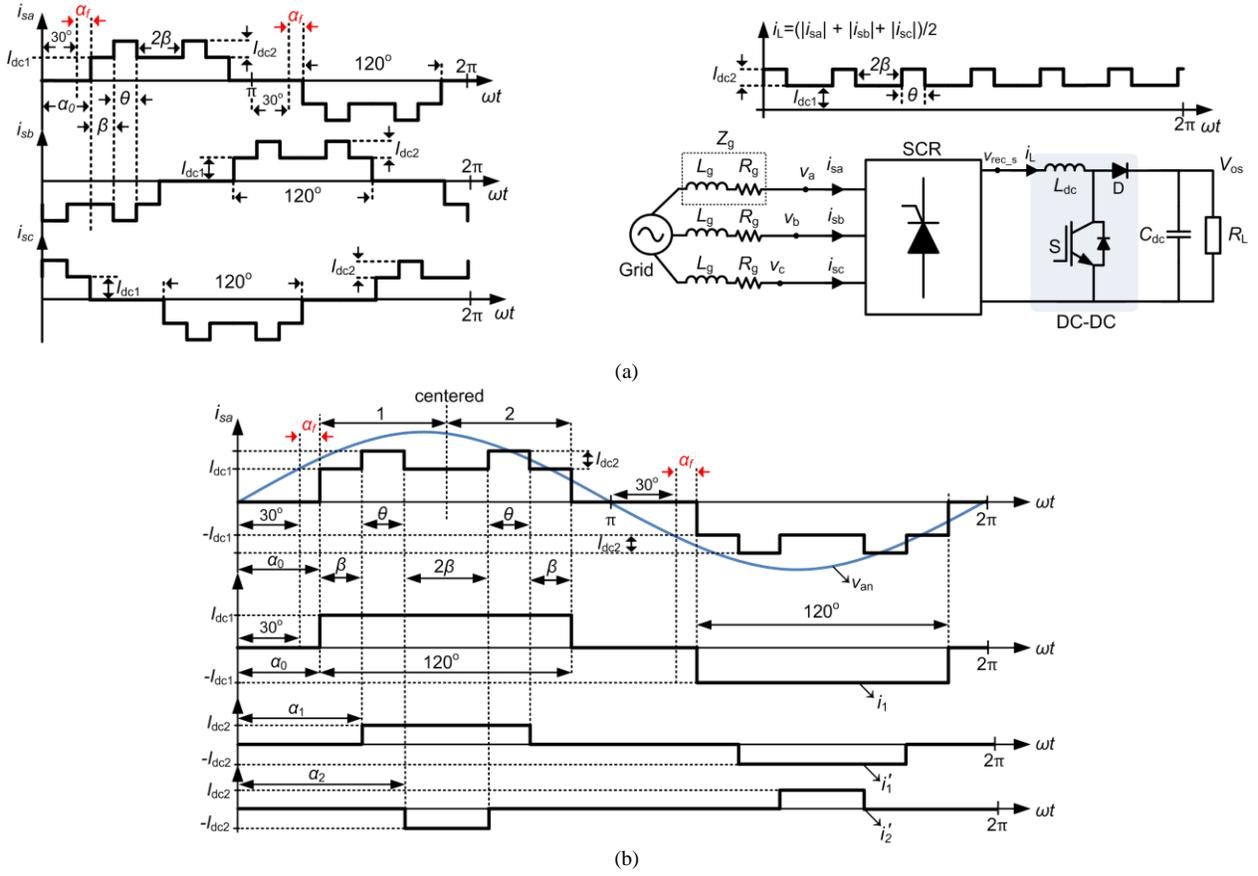
Fig. 4. Illustration of the proposed current modulation with selected harmonic cancellation: (a) typical waveforms in a SCR unit ( $\alpha_f = 0^\circ$  in the case of diode rectifiers) and (b) conceptual illustration of the proposed modulation scheme.
