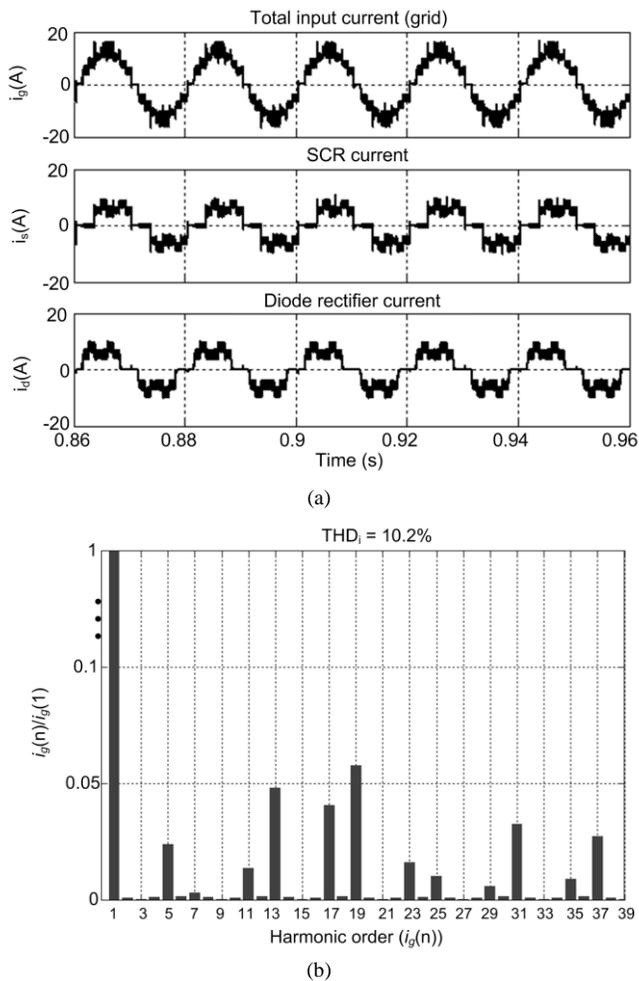
Fig. 10. Performance of the proposed method with current modulation when  $THD_i$  is optimized where the total power level is 5.5 kW: (a) current waveforms (phase a) and (b) spectrum of the low-order harmonics in the grid current.
