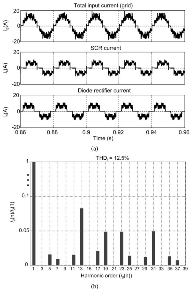
Fig. 9. Performance of the proposed method with current modulation when 5<sup>th</sup>, 7<sup>th</sup> and 11<sup>th</sup> harmonics are optimized for reduction where the total power level is 5.5 kW: (a) current waveforms (phase a) and (b) spectrum of the low-order harmonics in the grid current.
