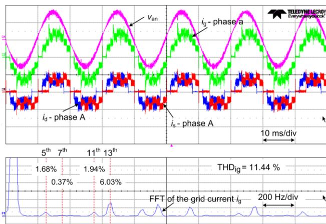
Fig. 16. Experimental results (phase a) of the multi-drive system with the novel current modulation scheme at  $P_{in} \approx 6$  kW,  $V_o = 700$  V, targeting at reducing the low order harmonics and also a lower  $THD_i$ ; grid current  $i_g$  [10 A/div], grid phase voltage  $v_{an}$  [200 V/div], diode rectifier input current  $i_d$  [10 A/div], SCR unit input current  $i_s$  [10 A/div], and Fast Fourier Transform (FFT) analysis of the grid current [500 mA/div].
