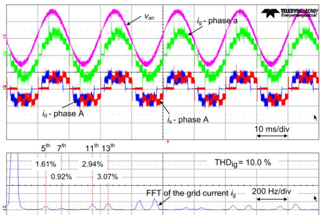
Fig. 17. Experimental results (phase a) of the multi-drive system with the novel current modulation scheme at  $P_{in} \approx 5.85$  kW,  $V_o = 700$  V, targeting at a minimized  $THD_i$ ; grid current  $i_g$  [10 A/div], grid phase voltage  $v_{an}$  [200 V/div], diode rectifier input current  $i_d$  [10 A/div], SCR unit input current  $i_s$  [10 A/div], and Fast Fourier Transform (FFT) analysis of the grid current [500 mA/div].
