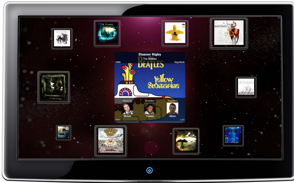
Figure 2: The situated display contains information about the current song playing in the center, surrounded by representations of nominated songs. The size of the nominations indicates current ranking, meaning that the largest nomination will be played next.
