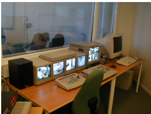
Figure 4. Control room: equipment for operating the motorized video cameras in the subject room.
