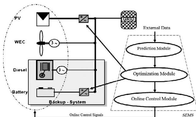
FIG. 3. SEMS in smart grid.
