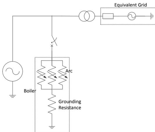
Figure 8 - Single-line diagram of the simulated system
