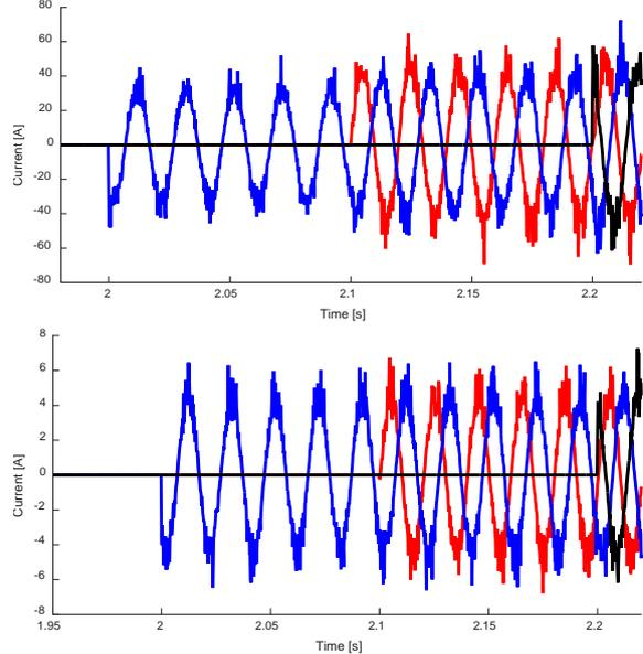
**Figure 11 - Current in the boiler for Cases 6 (up) and 3 (down). Switch-on: Phase A: 2s; Phase B: 2.1s; Phase C: 2.2s**
