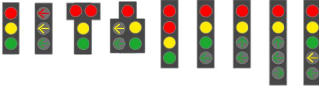
Fig. 3: Examples of vertical TLs found in California. [28]
