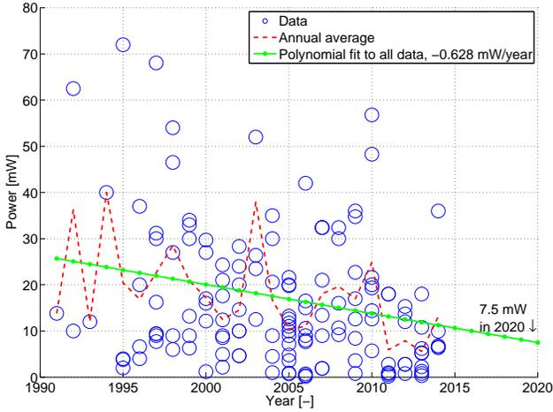
Fig. 2. LNA power consumption evolution.
