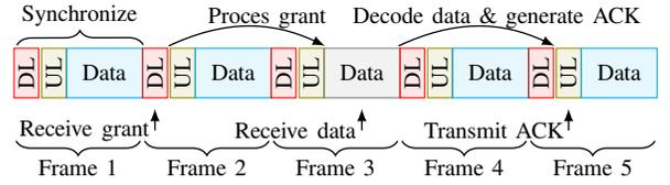
Fig. 2: Procedure for receiving data in 5G.
