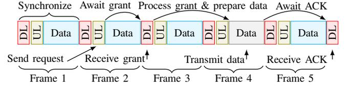
Fig. 4: Procedure for transmitting data in 5G.
