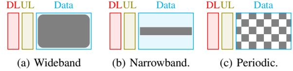
Fig. 8: Allocation of the wake-up signal (gray color).
