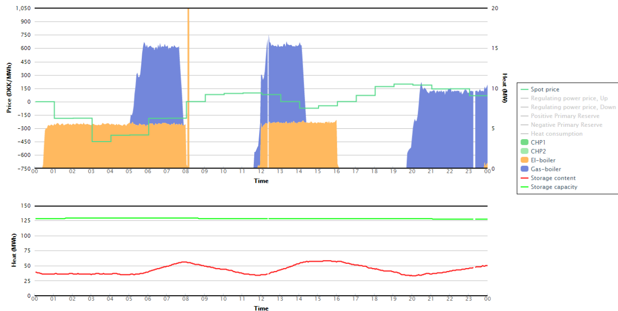
Figure 5: Operation of CHP unit, electric boilers, and thermal storage in Hvide Sande district heating plant (Denmark), in response to a low price on the electricity spot market ( www.emd.dk ). This demonstrates how thermal storage can be activated by low electricity prices, which often occur in hours of high wind penetrations.
