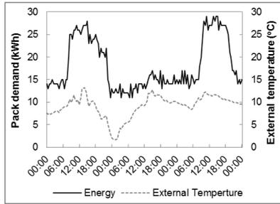
Fig. 6 Pack energy use and average external temperature from 07/04/2012 to 09/04/2012.
