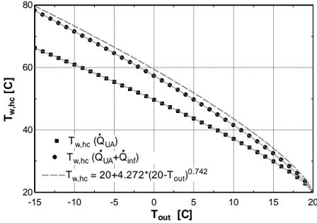
Fig. 2 Ideal v/s fitted heating curve temperature
