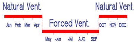
Fig.5 Façade cavity ventilation mood
