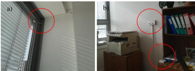
Fig. 6: a) window surface temperature sensor, b) illuminance sensor (bottom), air temperature, relative air humidity and CO<sub>2</sub> concentration sensor (top) in the office 609.
