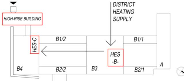
Fig. 3: Heat supply to the building and location of heat exchange stations (HES).
