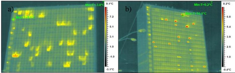
Fig. 2: a) Simple facade with triple glazing, facing North-West, b) Double skin facade, facing South-East. Photo: Michal Lukačovič
