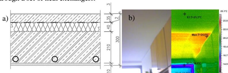
Fig. 4: a) detail of the ceiling structure, b) infrared image of the thermally active ceiling.
