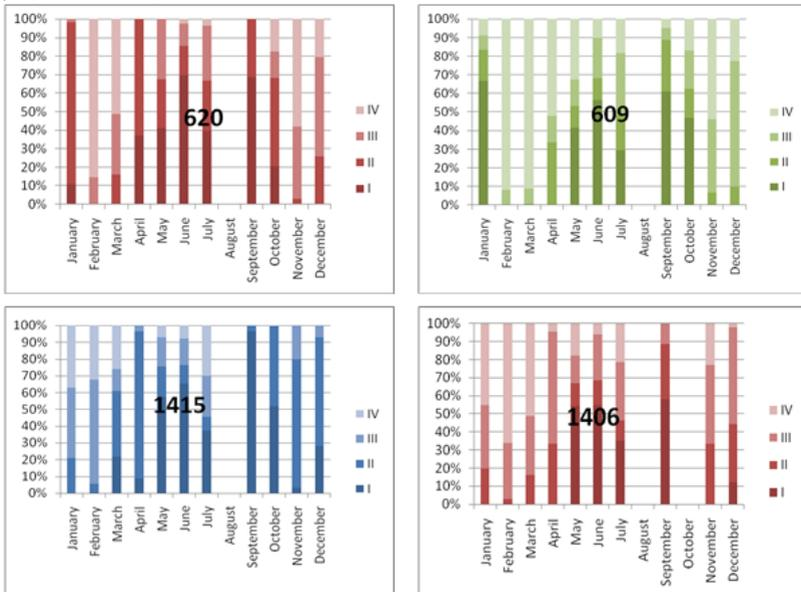
Fig. 7: Classification of thermal environment into 4 categories in accordance with EN 15251, 4 reference spaces of the high-rise building.
