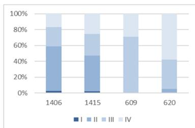
Fig. 10: Classification of the reference rooms according to the indoor air quality into 4 categories.
