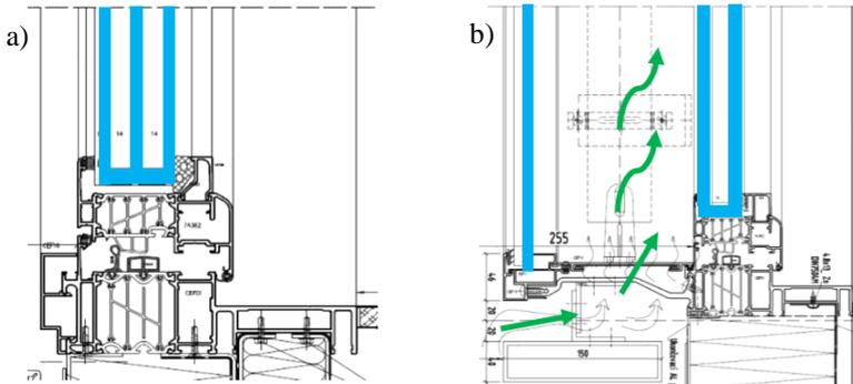
Fig 1: a) simple facade facing North-West, b) double skin facade facing South-East.
