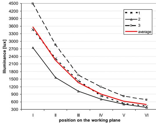
Fig. 5 Illuminance [lux] in the middle of the residential area between the glazed facade and the onyx wall (1 – 1<sup>st</sup> measurement, 2-2<sup>nd</sup> measurement, 3-3<sup>rd</sup> measurement, average – average value from 1,2 and 3)
