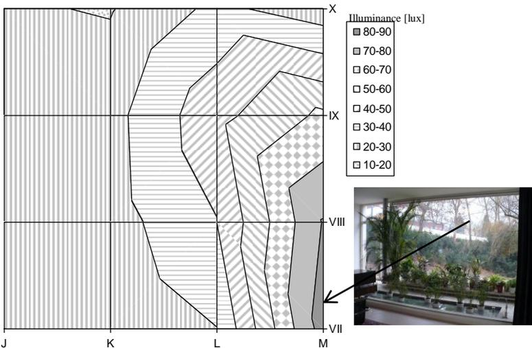
Fig. 8 Illuminance distribution on the working plane at the residential area outside of the onyx wall, J to M – VII to X (measurements for the mean external horizontal illuminance 7150 lux).
