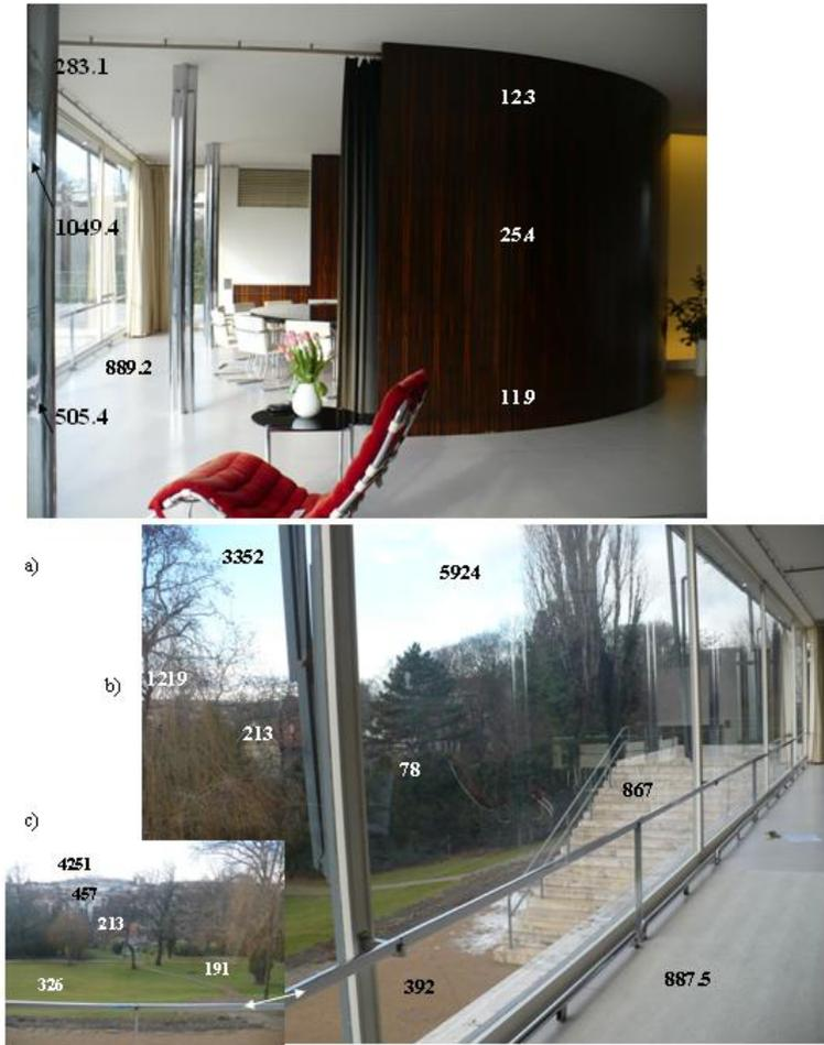
Fig. 12 Luminance [ $\text{cd}\cdot\text{m}^{-2}$ ] of surfaces in a view out of the onyx wall to the glazed area of the facade and the dark part of the internal wooden partition
