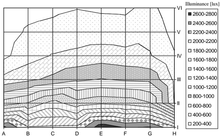
Fig. 6 Illuminance distribution on the working plane between the glazed facade and the onyx wall (the measurements for the mean external horizontal illuminance 7150 lux).
