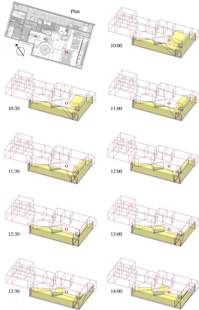
Fig. 13 Insulated area (yellow parts), 13<sup>th</sup> January from 10:00 to 14:00, (O – onyx wall)
