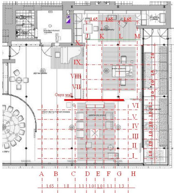
Fig. 3 Part of the ground floor residential area with the positions of illuminance measurements
