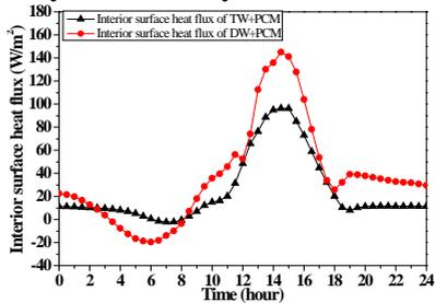
Fig. 9. The heat flux on the interior surface of the TW+PCM and DW+PCM in the sunny summer day
