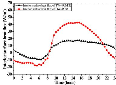
Fig. 11. The heat flux on the interior surface of the TW+PCM and DW+PCM in the rainy summer day
