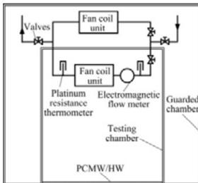
Fig. 4. Internal structure of the experimental chambers
