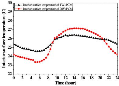
Fig. 10. The temperature on the interior surface of the TW+PCM and DW+PCM in the rainy summer day
