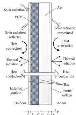
Fig. 2 Heat transfer process of the TW+PCM
