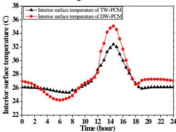
Fig. 8. The temperature on the interior surface of the TW+PCM and DW+PCM in the sunny summer day
