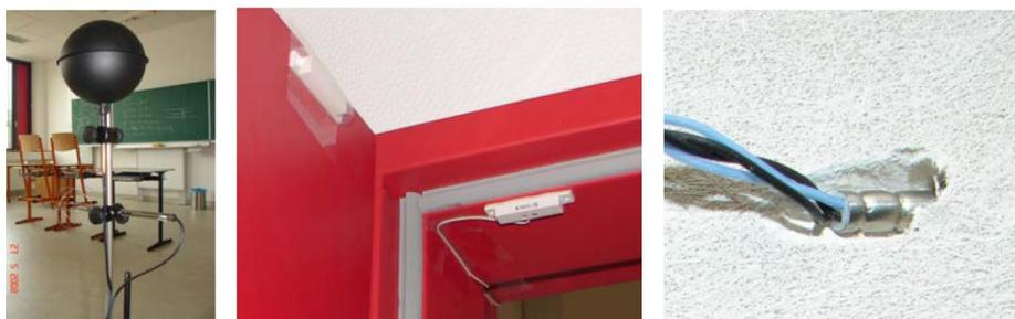
Fig. 1 left: operative room temperature, middle: reed contact door, right: wall center temperature sensor [7]
