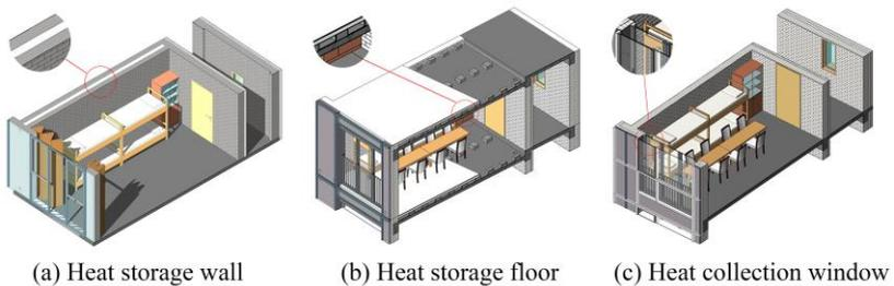
Fig. 8 Designs for heat collection and storage
