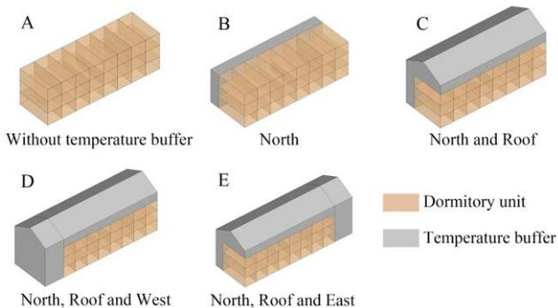
Fig. 4 Locations of temperature buffer for the dormitory
