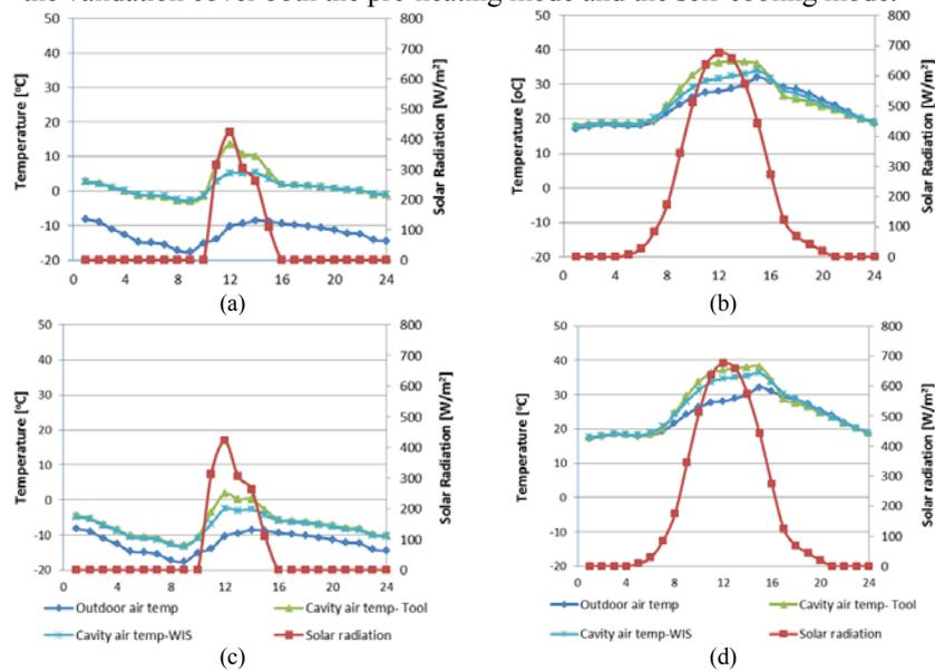
Fig. 6 Comparison of calculated cavity air temperatures by the developed Tool and WIS (a) Sample 1 in sunny winter (b) Sample 1 in sunny summer (c) Sample 2 in sunny winter (d) Sample 2 in sunny summer
