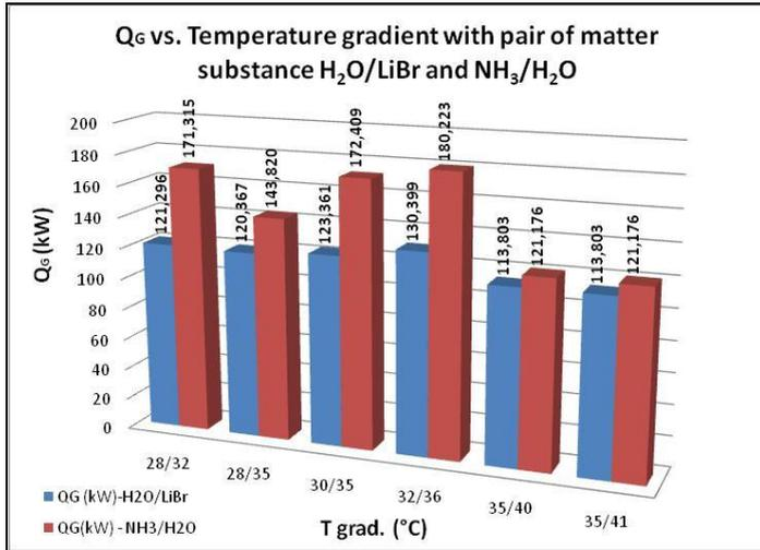
Fig. 5 Comparison  $Q_g$  vs. Temperature gradient working solution  $\text{H}_2\text{O}/\text{LiBr}$  and  $\text{NH}_3/\text{H}_2\text{O}$  depends on temperature gradient for absorber and condenser
