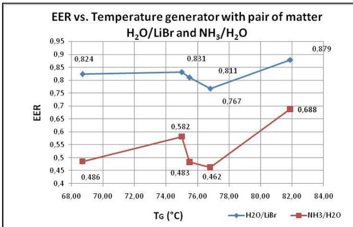
Fig. 4 Comparison EER vs. Temperature of generator working solution H<sub>2</sub>O/LiBr and NH<sub>3</sub>/H<sub>2</sub>O
