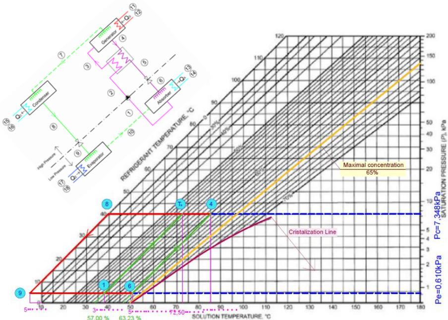
Fig. 3 Model of absorption cycle in P-x-T diagram with working substance H<sub>2</sub>O/LiBr [3]
