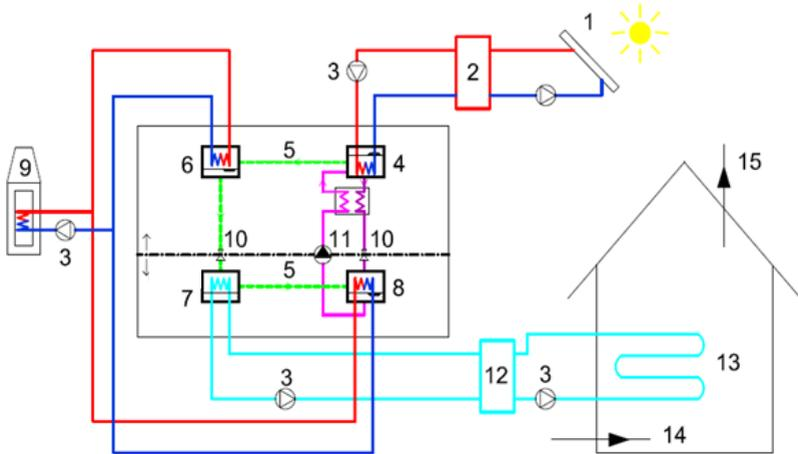
Fig. 1 The basic scheme of absorption cooling [9]
