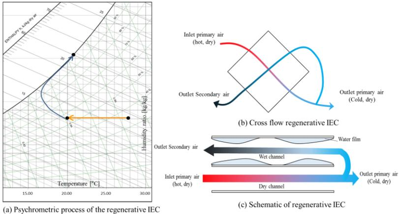
Fig. 2 Cooling process of regenerative indirect evaporative cooler
