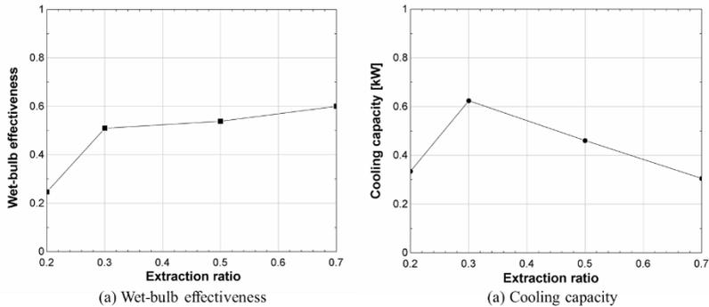
Fig. 5 Effects of extraction ratio in regenerative IEC
