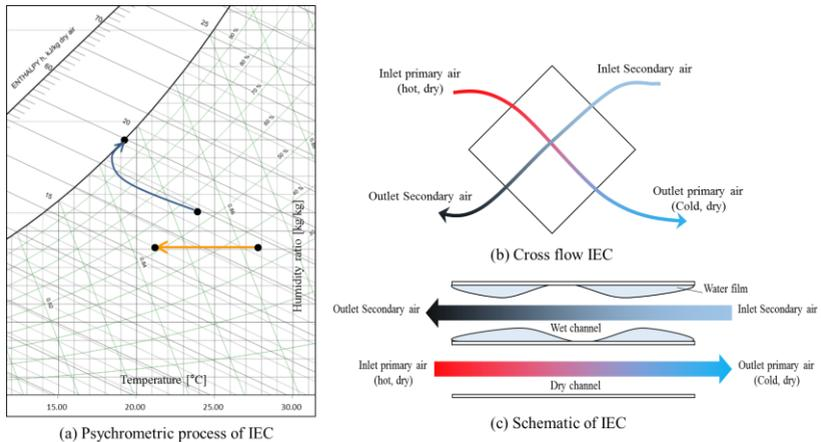
Fig. 1 Cooling process of indirect evaporative cooler
