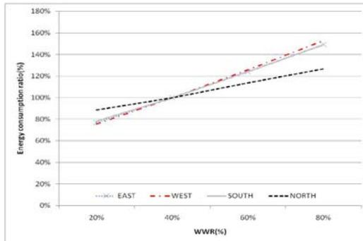
Fig. 2 Simulation Results by WWR and Orientation
