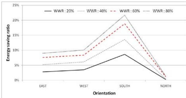
Fig. 4 Energy saving ratio by orientation and WWR
