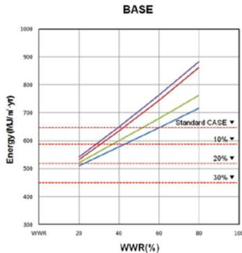
Fig. 5 Guideline by energy simulation results
