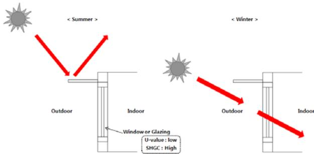
Fig. 1 Ideal concept of Shading & Window role
