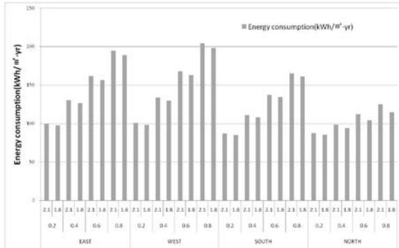
Fig. 3 Energy consumption by various performance factor and orientation
