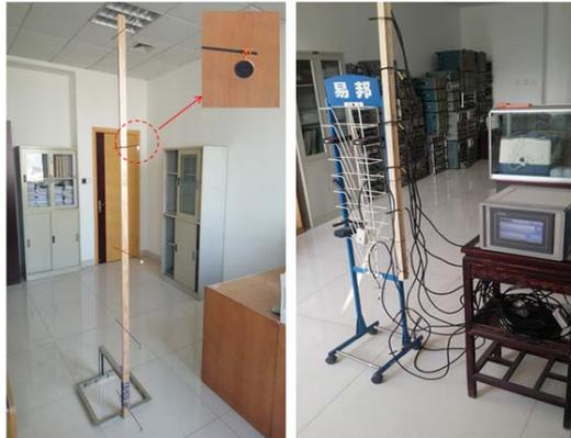
Fig. 3 Measured instruments for vertical temperature distribution
