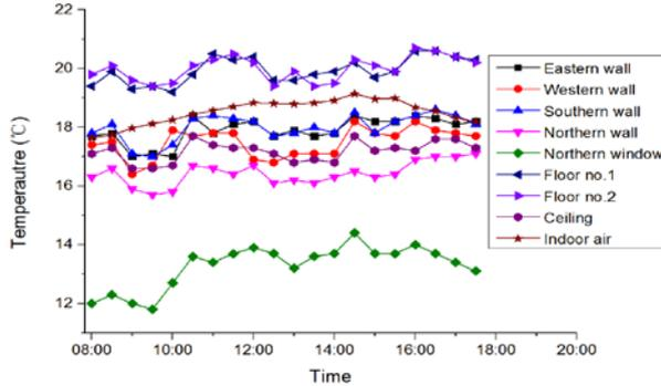
Fig. 4 Variation of indoor air and interior wall surfaces temperature in a northern room in the fifth floor in Dec. 29, 2015
