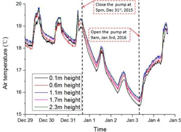
Fig. 5 Variation of indoor air temperature at the different height above the floor in a northern room in the fifth floor from Dec 29, 2015 to Jan 5, 2016
