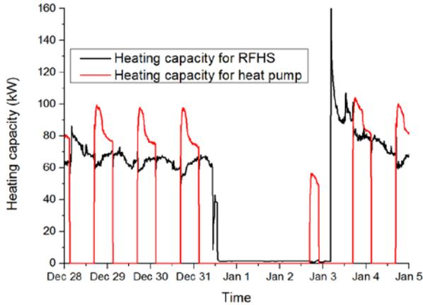
Fig. 6 Variation of heating capacity for radiant floor heating system and heat pump from Dec 29, 2015 to Jan 5, 2016
