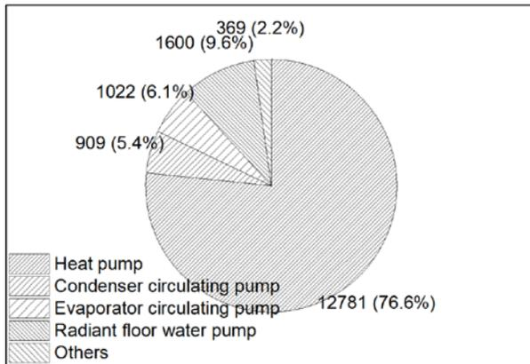
Fig. 7 Constitute for the energy consumption of radiant floor heating system from Dec 21, 2015 to Jan 20, 2016
