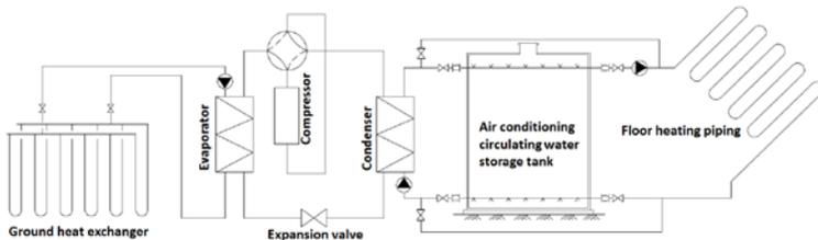
Fig. 2 System schematic diagram of the radiant floor heating system with ground source heat pump in winter
