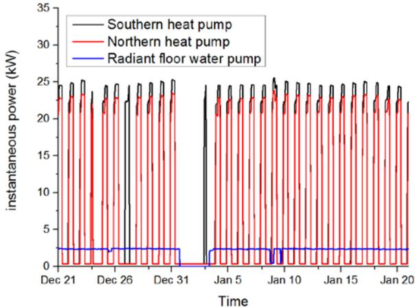
Fig. 9 Variation of instantaneous power for southern heat pump, northern heat pump and radiant floor water pump from Dec 21, 2015 to Jan 20, 2016
