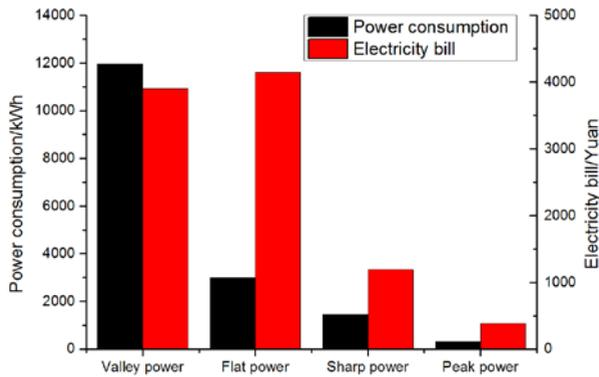
Fig. 8 Comparison of the power consumption and electricity bill for the radiant floor heating system from Dec 21<sup>st</sup>, 2015 to Jan 20<sup>th</sup>, 2016
