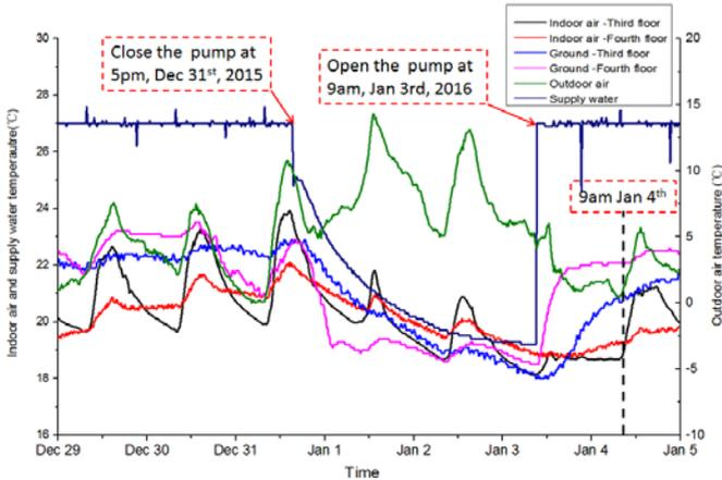
Fig. 10 Variation of indoor air temperature, floor surface temperature, outdoor air temperature and supply water temperature from Dec 29, 2015 to Jan 5, 2016
