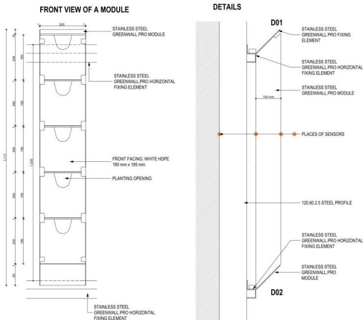
Fig. 1 The construction of the living wall panels and the places of the sensors
