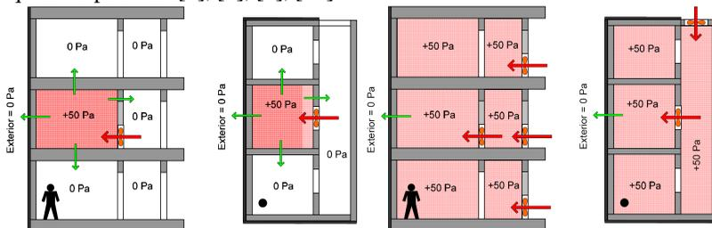
Fig. 1 Single zone test with adjacent zones open to exterior (two left figures: section and plan view of test floor) and guarded zone test with adjacent zones pressurized (right figures) [9]
