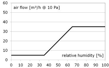
Fig. 3 Trickle vents air flow as a function of relative humidity characteristics by manufacturer
