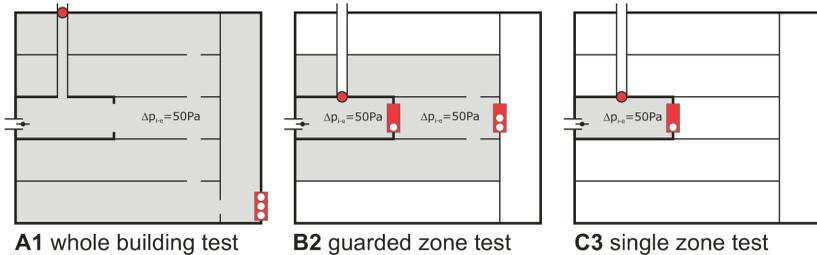
Fig. 6 Measurements configurations (pressurized zone marked with grey colour)
