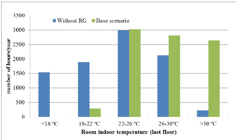
Figure 5 – Annual indoor temperature in one last floor bedroom without RG and in the base scenario (free-floating temperatures)
