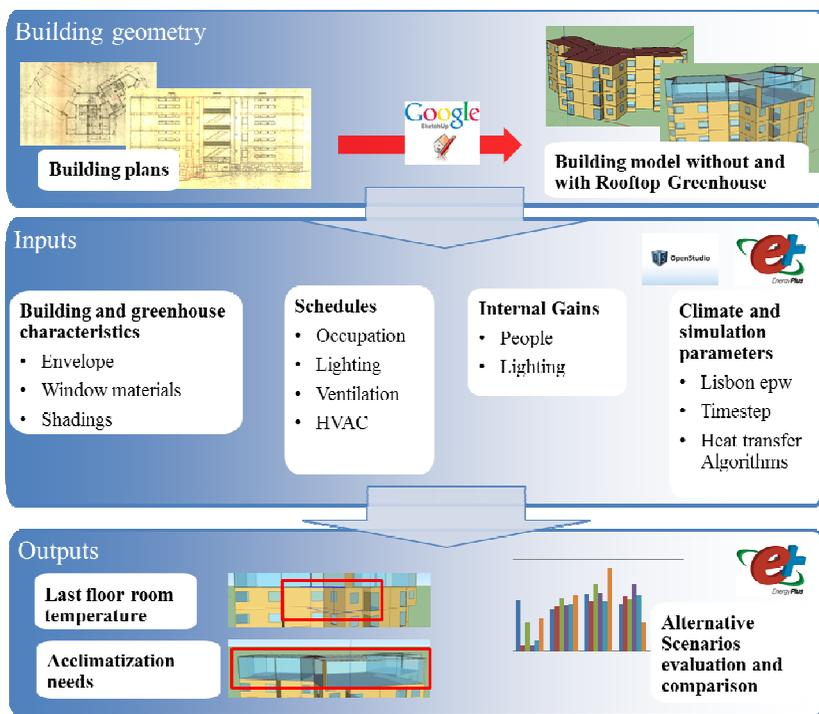
Figure 2 – Simulation methodology schematic
