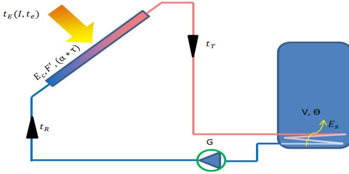
Fig. 2- Solar Collector circuit scheme
