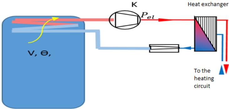
Fig. 3 – Supply system containing the heat pump
