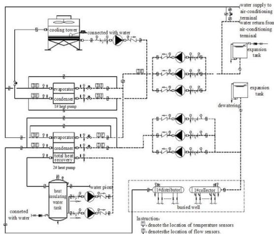
Fig. 1. Schematic diagram of the GSHP system
