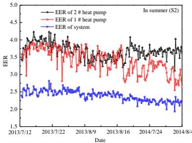
Fig. 10. EER of 1#heat pump, 2# heat pump and system in mode S2
