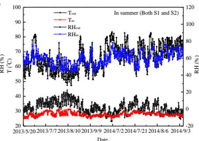
Fig. 3. Outdoor and indoor temperature and relative humidity in summer
