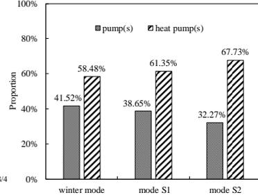
Fig. 11. Energy consumption proportions of pumps and heat pumps
