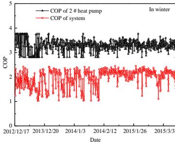
Fig. 8. COP of 2# heat pump and system in winter
