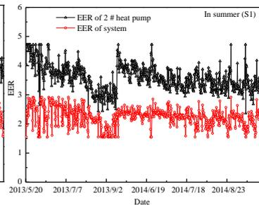
Fig. 9. EER of 2# heat pump and system in mode S1
