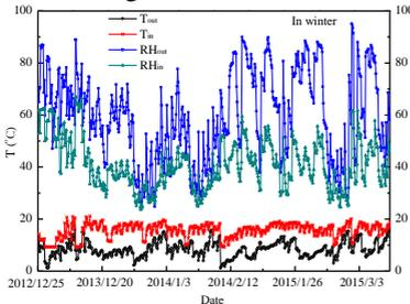
Fig. 2. Outdoor and indoor temperature and relative humidity in winter
