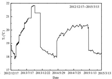
Fig.7. soil temperature in whole monitoring period
