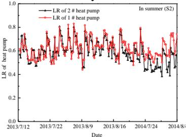
Fig. 6. LR of 1# heat pump and 2# heat pump in mode S2
