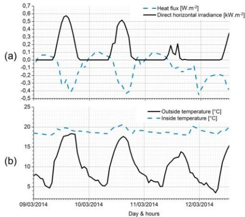
Figure 4 : (a) Heat flux in the southern wall against solar irradiance for March 2014; (b) Inside and outside temperature for March 2014
