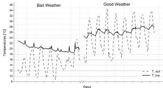
Figure 6 : Inside and outside temperatures for the two weeks referenced as "bad" and "good" weather during summer 2013
