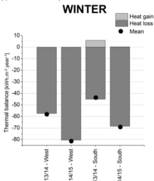
Figure 3 : Thermal balance of West and South walls in winters 2013/14 and 2014/15
