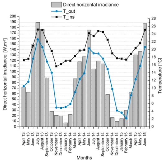
Figure 2 : Outside and inside temperatures and direct horizontal irradiance
