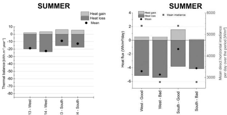
Figure 5 : (a) Thermal balance of West and South walls in summer 2013/14 and 2014/15 ; (b) Daily thermal balance for good (GW) and bad (BW) weathers of West and South walls in summer 2013
