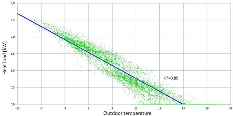
Fig. 2 Heat power required by the building as a function of the external air temperature. The blue line is the linear regression (i.e. Building Energy Signature).
