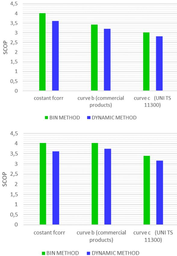
Fig. 3 Seasonal performance of two different HP sizes (i. e. thermal power): 80% of design load (above) and 60% of the design load (below). Calculation with bin method and dynamic method.
