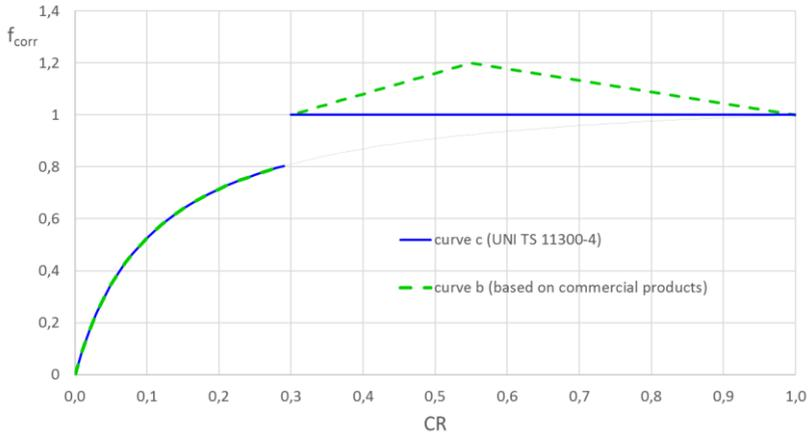
Fig. 1 COP degradation functions at part load. The  $CR$  value where the  $COP$  begins to degrade (here, 0.3) and the  $CR$  value where the maximum of  $f_{corr}$  occurs (0.55), as well as the maximum  $f_{corr}$  (1.2), can be modified as parameters of the Type, depending on the specific performance of the unit.
