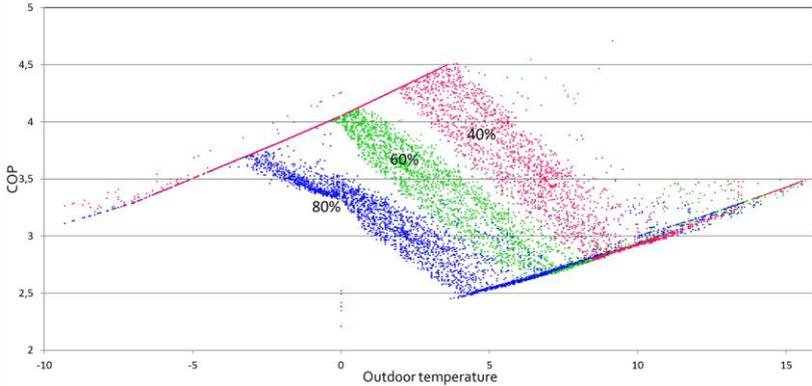
Fig. 5 COP for different heat pump size (percentage of rated power over design heat load) depending on outdoor temperature.
