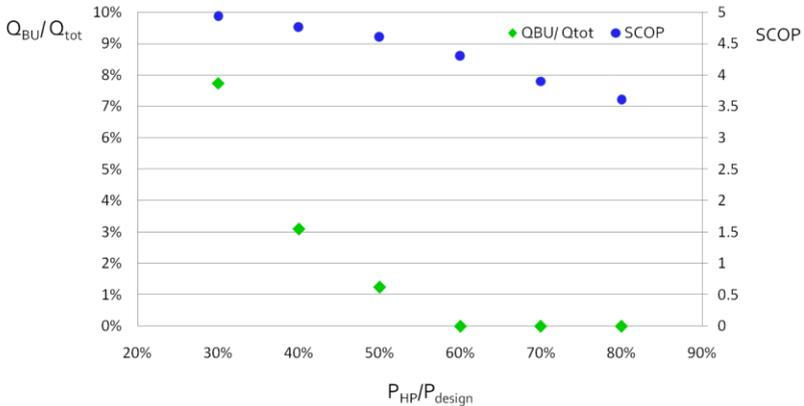
Fig. 6 SCOP and backup heat percentage for different HP sizes.
