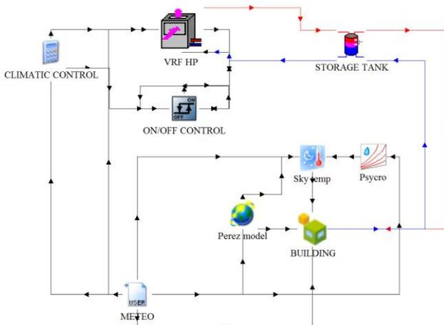
Fig. 4 Building and heating system model (TRNSYS)
