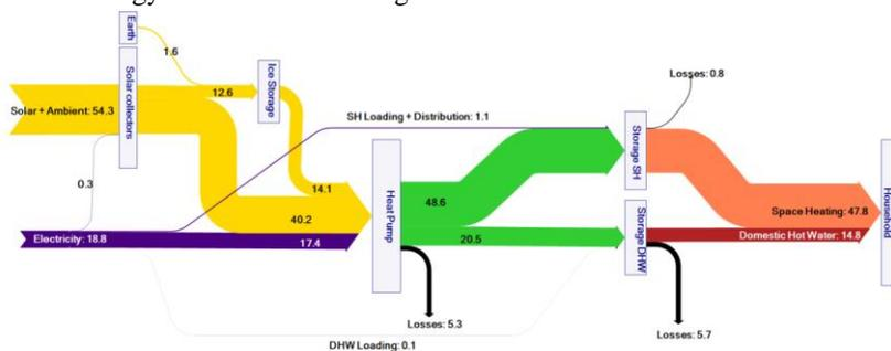
Fig. 5 Annual sankey-diagram for SFH45\* with solar ice storage heat pump system
