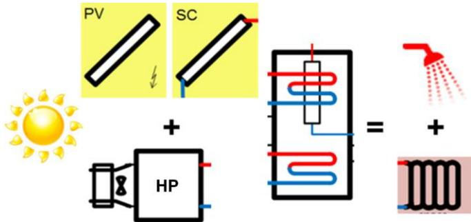
Fig. 1 Interaction of solar technology with heat generation and usage
