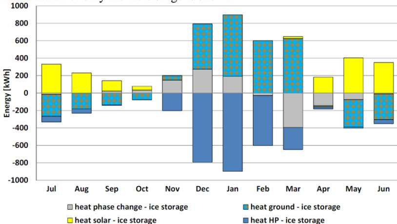
Fig. 7 Monthly energy balance of the ice storage of simulation SFH45\*. Heat exchange is depicted on the ordinate axis, subdivided into the different energy ratios. Positive values
