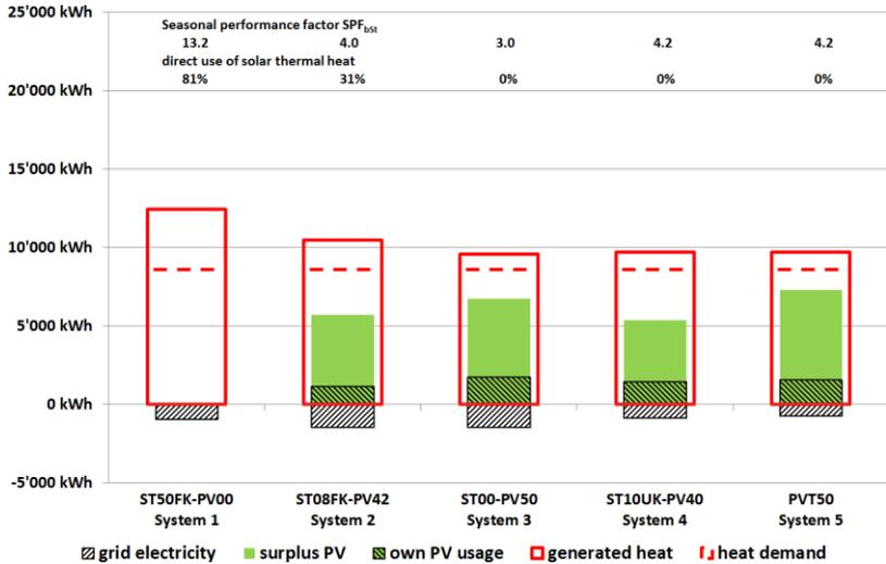
Fig. 2 Energy balance of five solar heat pump systems for SFH45
