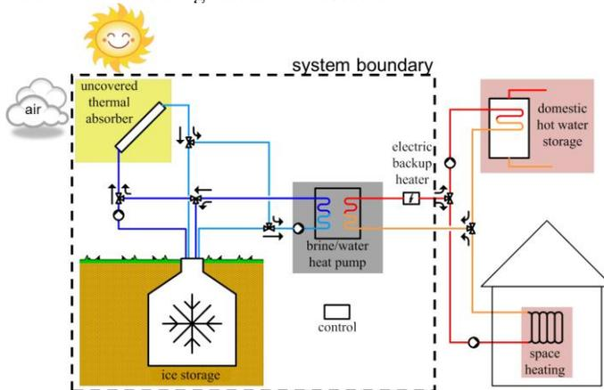
Fig. 4 Solar ice storage system hydraulics and evaluation boundary for  $SPF_{bSt}$
