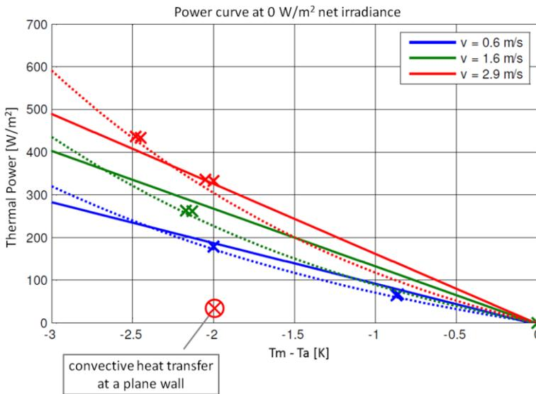
Fig. 8 Thermal power curves for test without irradiance and three different wind speeds. Measurement points are marked with an 'x', dashed lines indicate a polynomial fit and the results from the simulation model are shown as solid line.
