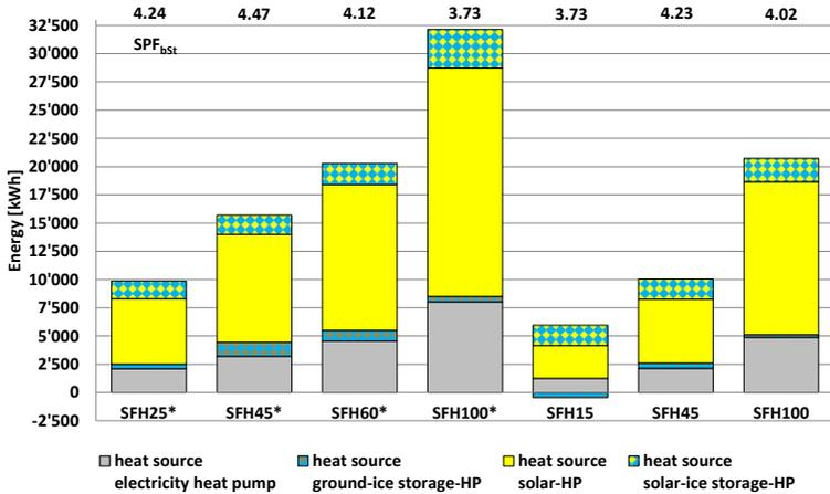
Fig. 6 Annual energy balance of the heat generations heat sources (heat pump, solar absorber and ice storage)
