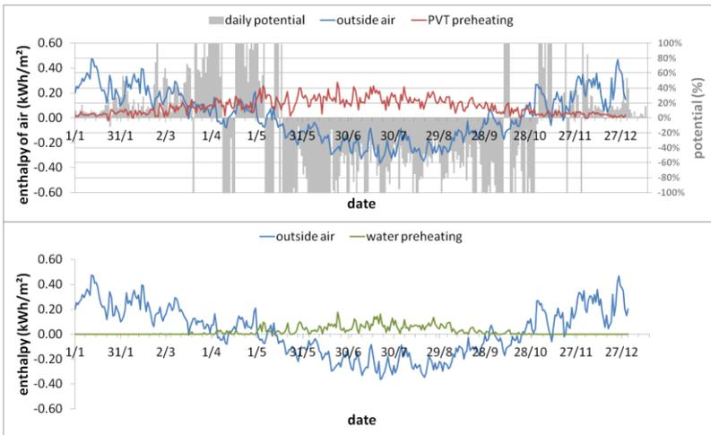
Fig. 5. Daily enthalpy change of the wine warehouse attributed to the continuous replacement of air with the exterior air. Top: potential of preheating injected air using the PVT array. Bottom: potential of preheating water using an air-water heat exchanger mounted on the roof.
