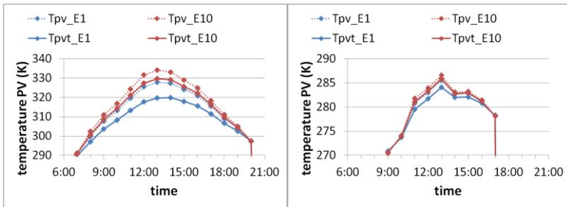
Fig. 4. Hourly temperature of ventilated (PVT) and PV branches during a summer (left) and a winter (right) day. Labels E1 and E10 represent the first and last modules of a branch.
