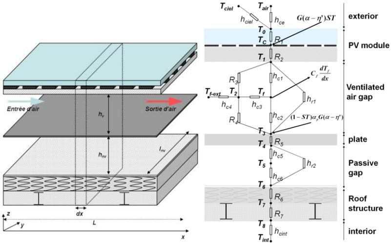
Fig. 2. Left: Simplified geometry of iNovaPVT structure shown discretisation in one dimensional slices. Right: Resistive network considered by the numerical model.
