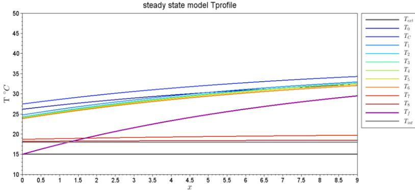
Fig. 3. Variation in steady state node temperatures along a single 9 m long ventilated branch for an incident solar radiation intensity of 500 W/m<sup>2</sup>.
