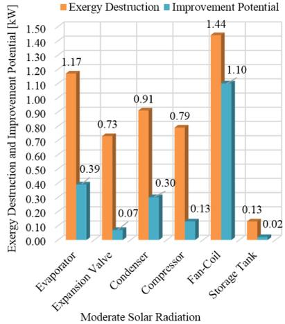
Fig. 5 Exergy destruction and improvement potential rates of each component of the system for moderate solar radiation
