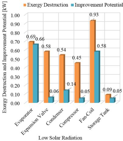
Fig. 4 Exergy destruction and improvement potential rates of each component of the system for low solar radiation
