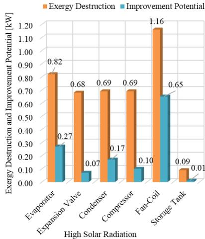
Fig. 6 Exergy destruction and improvement potential rates of each component of the system for high solar radiation
