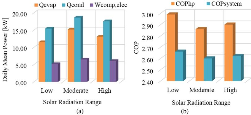
Fig. 3 Change of daily mean power rates of evaporator, condenser and compressor (a) and heat pump and overall system COP values (b) with different solar radiations
