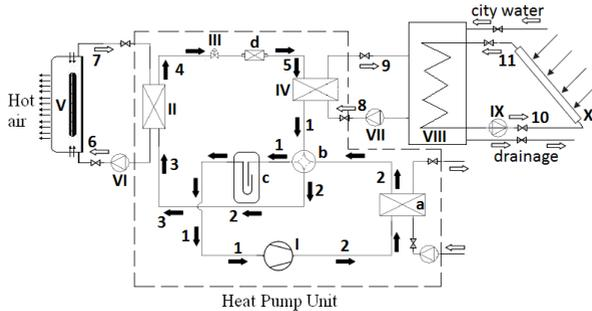
I: Compressor, II: Condenser (1) for air-conditioner, III: Expansion valve, IV: Evaporator
