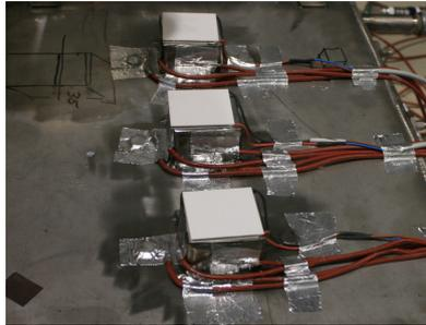
Fig. 2 Prototype 2 with cold water storage, the three extruded blocks, temperature measurement and the Peltier elements
