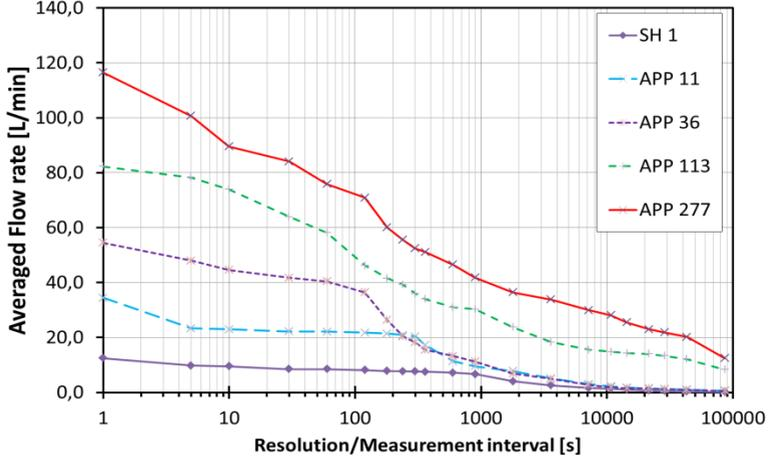
Figure 3: Peak flow rate,  $F$ , as a function of resolution,  $x$  for 5 different buildings with a centralized hot water installation, i.e. a single home (SH1) and 4 collective buildings with each a different number of flats (APP 11, APP 36, APP 113 and APP 227).
