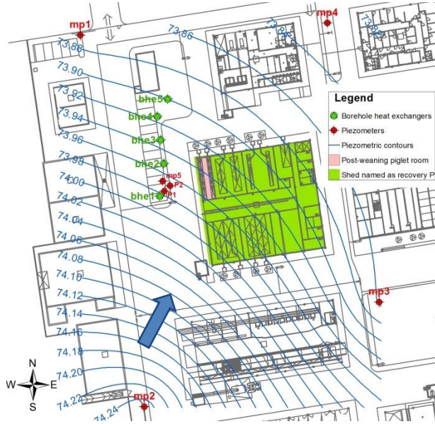
Fig. 2. Location of the piglets room, of the borehole field, of the piezometers and micro-piezometers. The groundwater flow direction is shown by the arrow.
