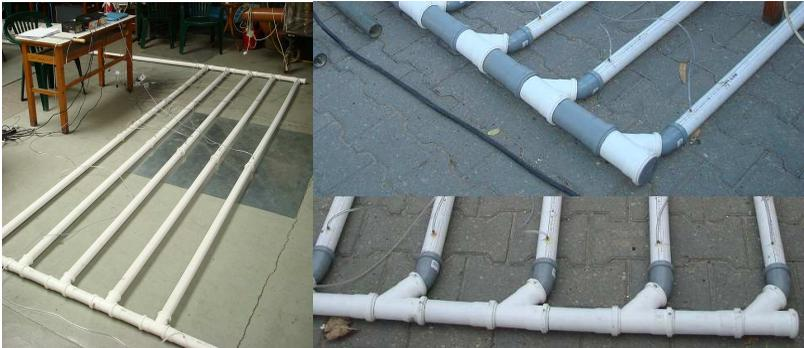
Fig. 4 The view of the exchanger model with the connection angle 90° (left photo) and 2x45° (right photo)
